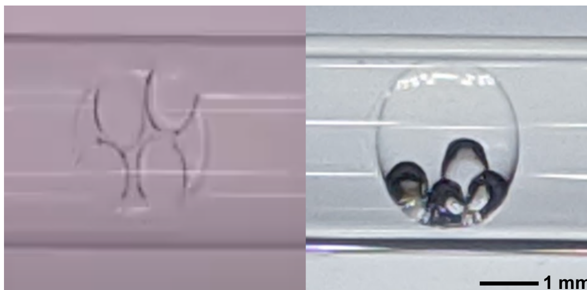
Fig. S2. Multicompartmental double emulsion images. Representative image of a tetra-compartmental double emulsion when taken from above with a stereomicroscope (left image). Representative image of the same tetra-compartmental double emulsion when taken from the side using a smartphone camera (right image). Images are unedited. Scale applies to both images.
