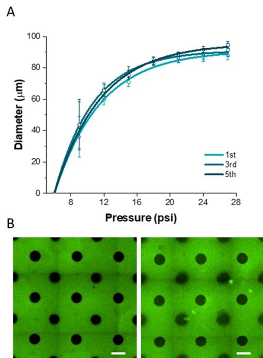
**Fig. S8** The reusability analysis of the SLB patterning chip. (A) A relation between applied pressures and average button diameters of the pattern after 5 consecutive uses of the same chip. (B) Fluorescence images of the hybrid SLB array formed using a fresh (left) and a reused chip (right). Scale bar is 100  $\mu\text{m}$ .
