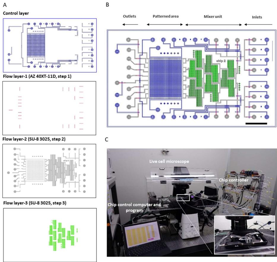
**Fig. S1** The design layout of the SLB patterning chip. (A) The control layer used 1 photomask while the flow layer used 3 photomasks for the mold fabrication. (B) A combined view of the patterning chip. Scale bar is 5 mm in B. (C) The chip control system on the fluorescence microscopy equipped with a live cell incubator system. The inset shows a zoom-in image of a mounted chip.
