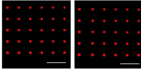
**Fig. S6** Lipid exchange between SLB patterns can be blocked in the absence of a diffusion barrier by using DPPC as constituent lipids. Fluorescence images of button SLB taken immediately (left) and 10 hours after (right) SLB formation; Lipid composition for the exterior area: 50% DPPC/50% Egg-PC, and for button area: 100% DPPC (doped with 0.01% Texas Red DHPE for visualization). Scale bar is 500  $\mu\text{m}$ .
