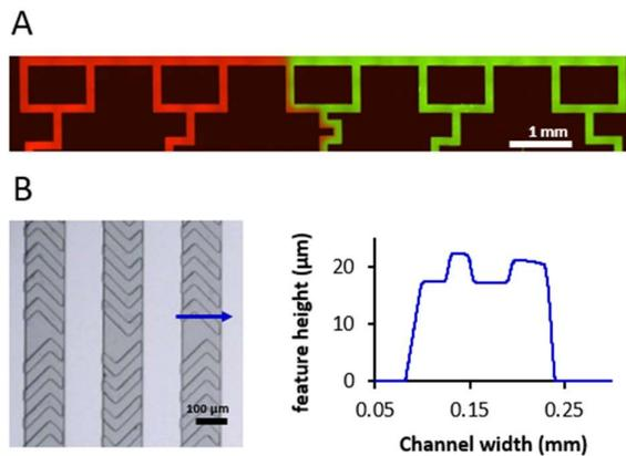
**Fig. S3** Optimization of the SUVs mixing by adding the staggered herringbone mixers (SHMs). (A) A fluorescence image of incompletely mixed SUVs. (B) A bright-field image (left) and the characterized height of SHMs at  $\sim 4\text{-}5\ \mu\text{m}$  measured by a stylus profilometry.
