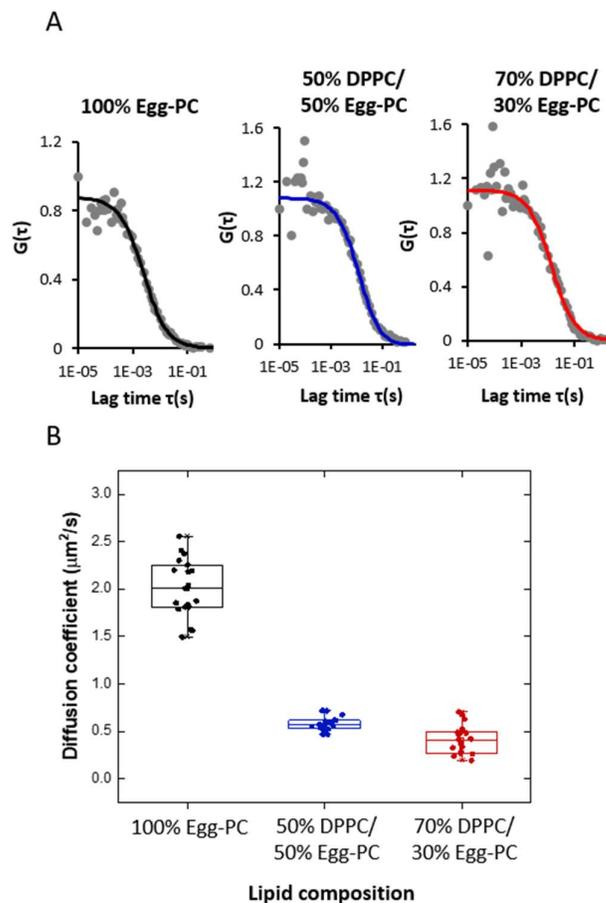
**Fig. S4** (A) Autocorrelation curves measured by the FCS and (B) resulting diffusion coefficients for SLB samples with lipid compositions of 100% Egg-PC (left), 50% DPPC/50% Egg-PC (middle) and 70%DPPC/30% Egg-PC (right) respectively.
