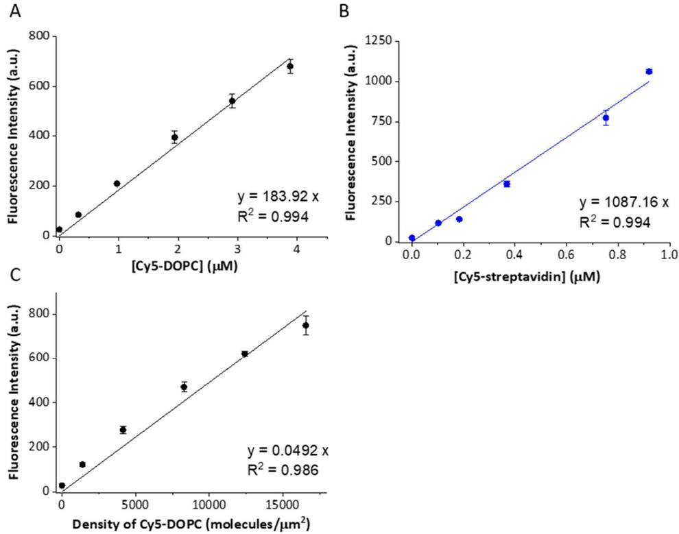
**Fig. S2** The density of Cy5-streptavidin on the SLB was measured using the quantitative fluorescence microscopy. (A) Cy5-doped vesicles were used as a bulk calibration standard. (B) A calibration plot showing fluorescence intensities of solutions containing labeled Cy5-streptavidin. (C) A series of Cy5-DOPC doped SLB were used as a surface density calibration standard.
