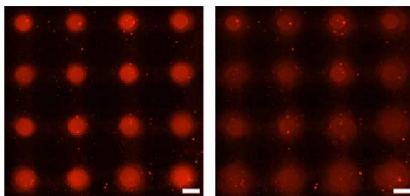
**Fig. S5** Significant lipid exchanges between patterned SLB was observed in the absence of the diffusion barrier. Fluorescence images of button SLB taken immediately (left) and 1 hours after (right) SLB formation; Lipid composition for the exterior area: 50% DPPC/50% Egg-PC, and for button area: 100% Egg-PC (doped with 0.01% Texas Red DHPE for visualization). Scale bar is 100  $\mu\text{m}$ .
