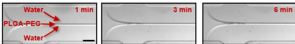
Figure S5. Microchannel images showing the macroscopic nanoprecipitation evolution of PLGA 10K -PEG 5K at 10 mg/mL by a 2D HFF device. With increasing time from 1 to 6 min, the device always worked well without polymer aggregation. This result demonstrates that hydrophilic PEG can effectively prevent polymer aggregation. Scale bar: 200 \mu m.
