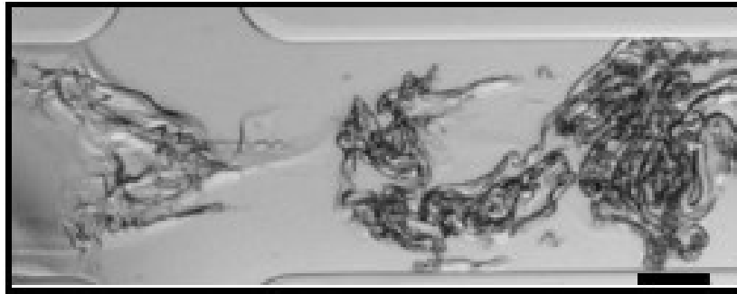
Figure S6. Microchannel images showing the polymer aggregation for PLGA 50K -PEG 5K at 90 mg/mL at 30 s operation. Scale bar: 200 \mu m.
