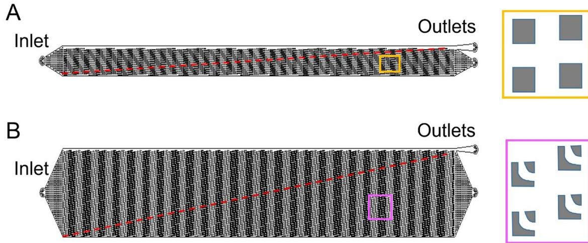
**Fig. S2.** Schematic chip designs of deterministic lateral displacement (DLD) structures. (A) Rectangular micro-post DLD design, (B) Filter-DLD design. The two structures have the same micro-post side length, gap width, and critical separation size ( $D_c$ ). Red dotted lines indicate inclination angles of micro-posts.
