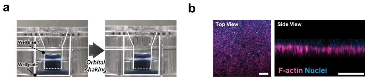
**Fig. S4** (a) Dye dispersion test on the 24-well plate of conventional Transwell system with orbital shaking. (b) Immunofluorescence images of Caco-2 intestinal epithelium cultured on orbitally shaken 24-well plate. The cells were stained with F-actin (magenta) and nuclei (cyan) (Scale bar: 50  $\mu$ m).
