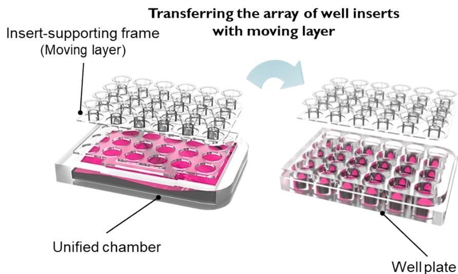
**Fig. S2** The moving layer of the insert-supporting frame allowed the easy transferring of well inserts from the unified chamber of BASIN to the conventional well plate.
