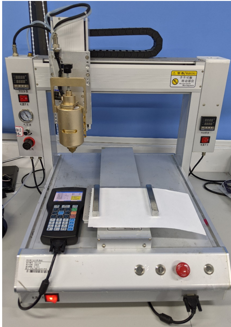
Figure S2 The automatic dispenser for PDMS wall printing.
