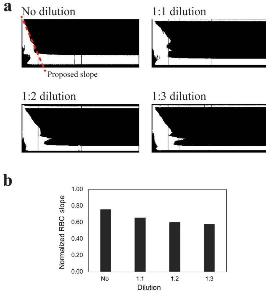
Figure S3. A proposed image analysis process using (a) Huang threshold and (b) normalized RBC slope with dilution factors. To analyze the orthogonal view images, the images are first converted to 8 bit using ImageJ with the default “Huang” setting selected to convert the images into black and white. The slope of the images is also calculated using ImageJ.
