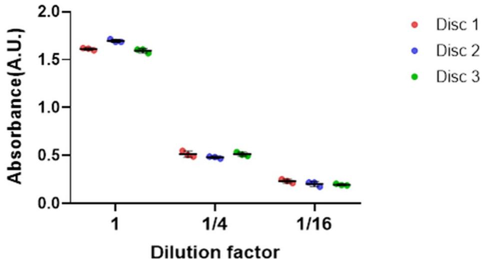
**Figure S4.** Disc-to-disc reproducibility of measuring the absorbance of a food dye at different concentrations with three different discs (n=3). C.V.(%) at different concentrations are 3.25%, 4.58%, and 8.73%, respectively.
