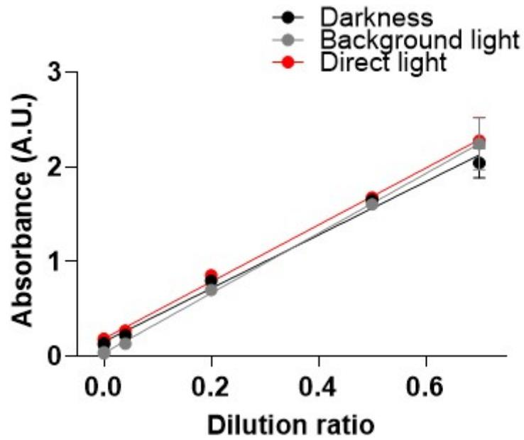
**Figure S2.** Robustness of the infrared sensor in three different light conditions measuring the optical density of a food dye at different dilution ratios.
