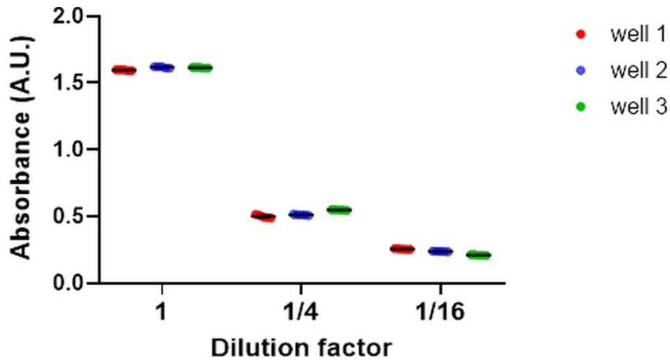
**Figure S3.** Well-to-well reproducibility of measuring the absorbance of a food dye at different concentrations in three different wells ( $n=5$ ). C.V.(%) at different concentrations are 0.63%, 4.35%, and 8.32%, respectively.
