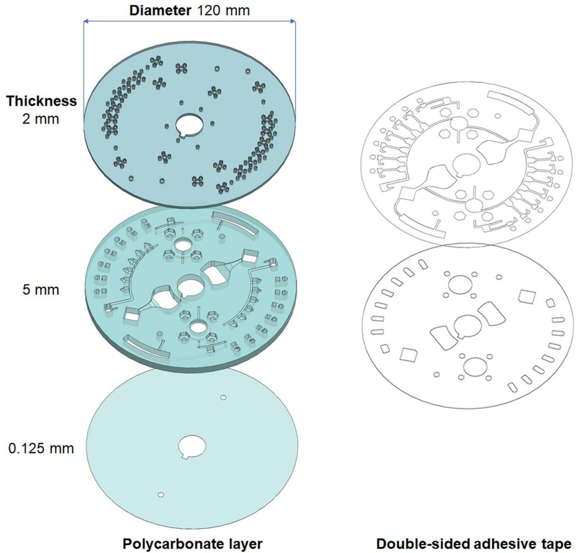
**Figure S1.** Device assembly (the top, middle, and bottom layers of the computer-numerical control (CNC)-milled polycarbonate layers with the double-sided adhesive tape in between).
