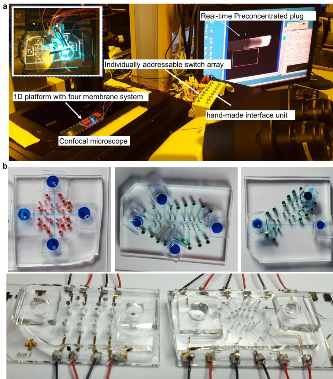
Fig. S1 (a) Experimental setup for digital control of a serial membrane system for actuation of the different membranes and (b) images of the different fabricated microfluidic platforms. The inset photo in (a) shows the external platinum electrodes introduced into a 2D channel geometry system.
