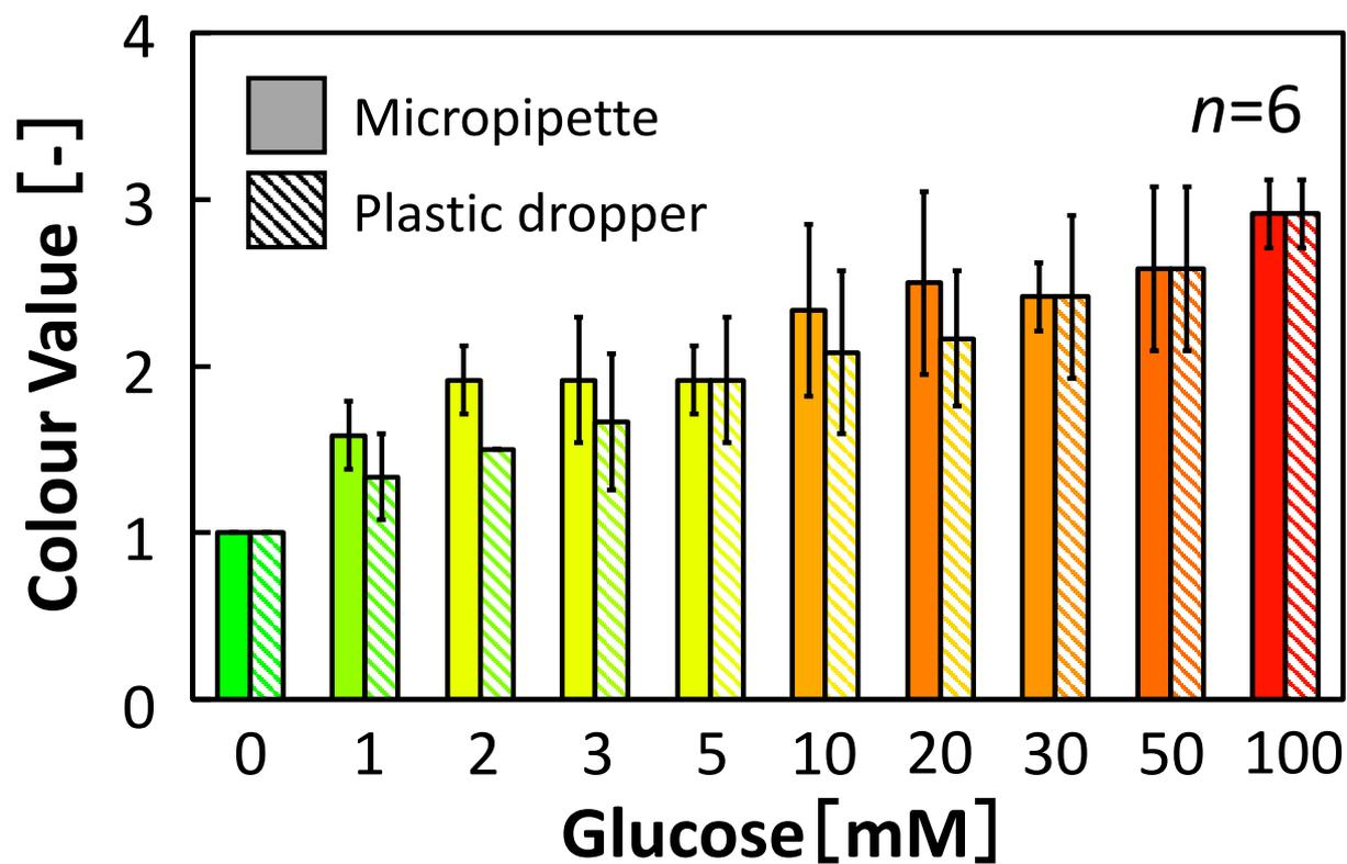
**Fig. S16** : Results of traffic light assay for glucose detection using Device 3 in combination with different sample application methods (micropipette or simple plastic dropper); error bars represent the mean values  $\pm 1\sigma$  ( $n = 6$ ).
