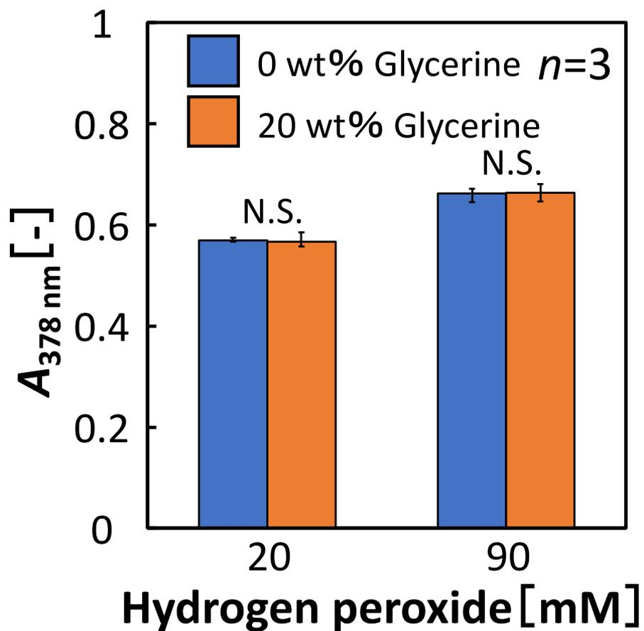
**Fig. S13** : Absorbance measurements after exposing paper disks modified with boronic acid pinacol ester for 20 min to solutions of  $\text{H}_2\text{O}_2$  in glycine buffer (pH 9.0) containing glycerine; error bars represent mean values  $\pm 1\sigma$  ( $n = 3$ ); N.S.: not significant.
