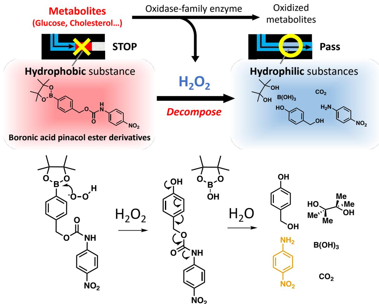
**Fig. S1** : (a) Chemical valving system using a boronic acid pinacol ester derivative as phase-switching substance: the hydrophobic state stops the sample flow, while the hydrophilic state induced by decomposition following reaction with  $H_2O_2$  allows the sample to flow through; (b) Mechanism of chemical decomposition of boronic acid pinacol ester derivative by reaction with  $H_2O_2$ , producing the yellow p-nitroaniline compound.
