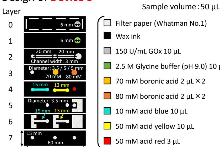
**Fig. S3** : Design details of various traffic light type  $\mu$ PADs: (a) Device 1, (b) Devices 2a, 2b, (c) Device 3. The indicated scales represent the pre-set values in the Adobe Illustrator CC software.
