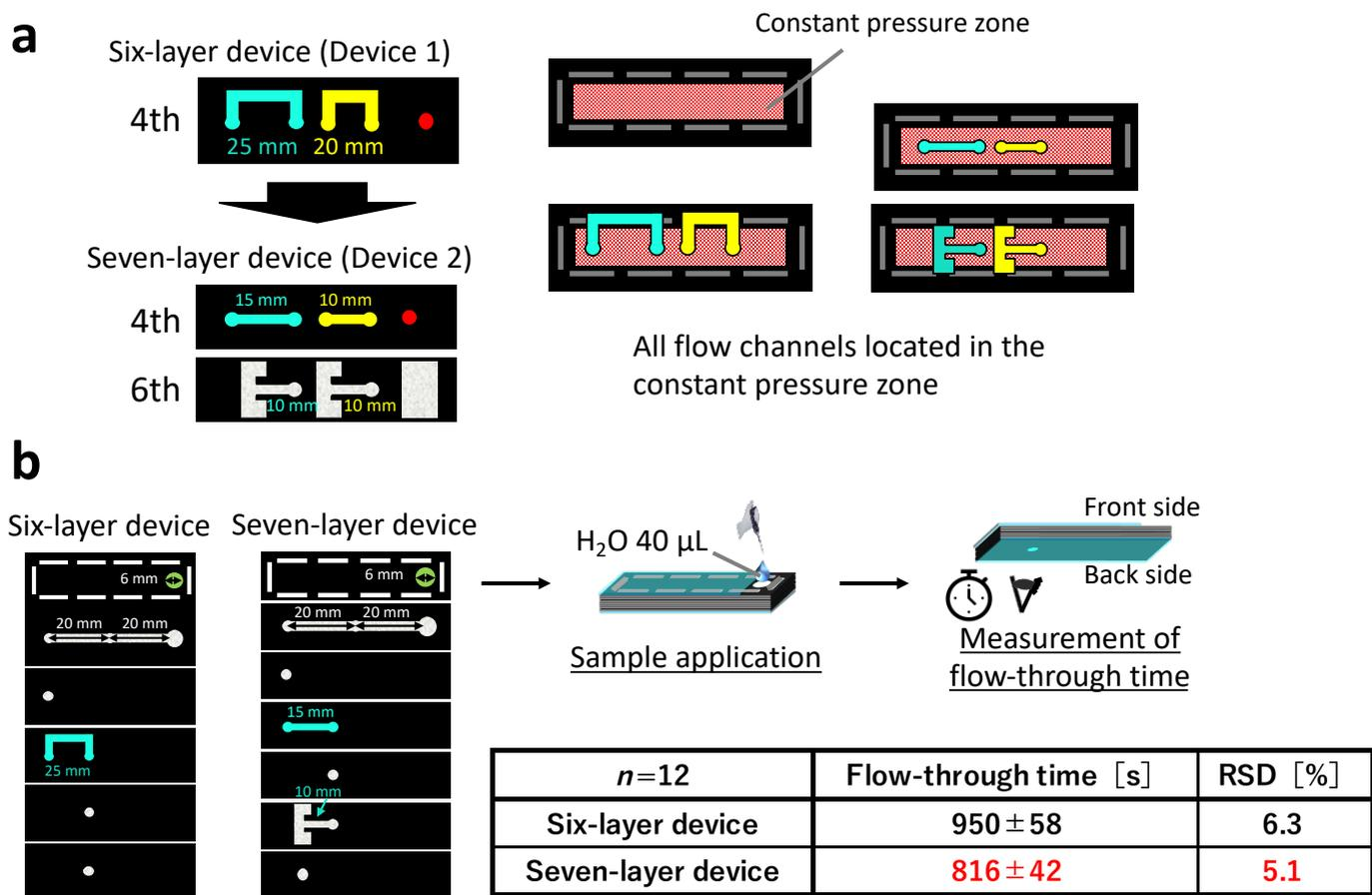
**Fig. S9** : Schematic illustration of flow channel modifications for device optimization: (a) Splitting of flow channels to arrange them in a zone of constant pressure (marked in red) between folded paper layers surrounded by staples; (b) outline of six- and seven-layer model devices (no hydrophobic walls; only green channel) used to measure the overall liquid flow-through times (mean  $\pm 1\sigma$  for  $n = 12$ ).
