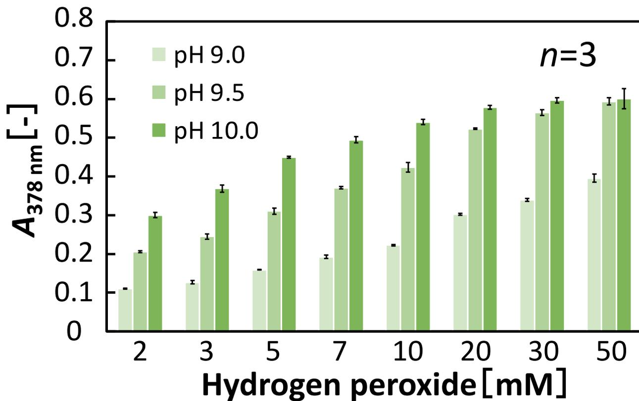
**Fig. S10** : Absorbance measurements after exposing paper disks modified with boronic acid pinacol ester for 10 min to solutions of various H<sub>2</sub>O<sub>2</sub> concentrations and different pH in glycine buffer (pH 9.0, 9.5, 10.0); error bars represent mean values  $\pm 1\sigma$  ( $n = 3$ ).
