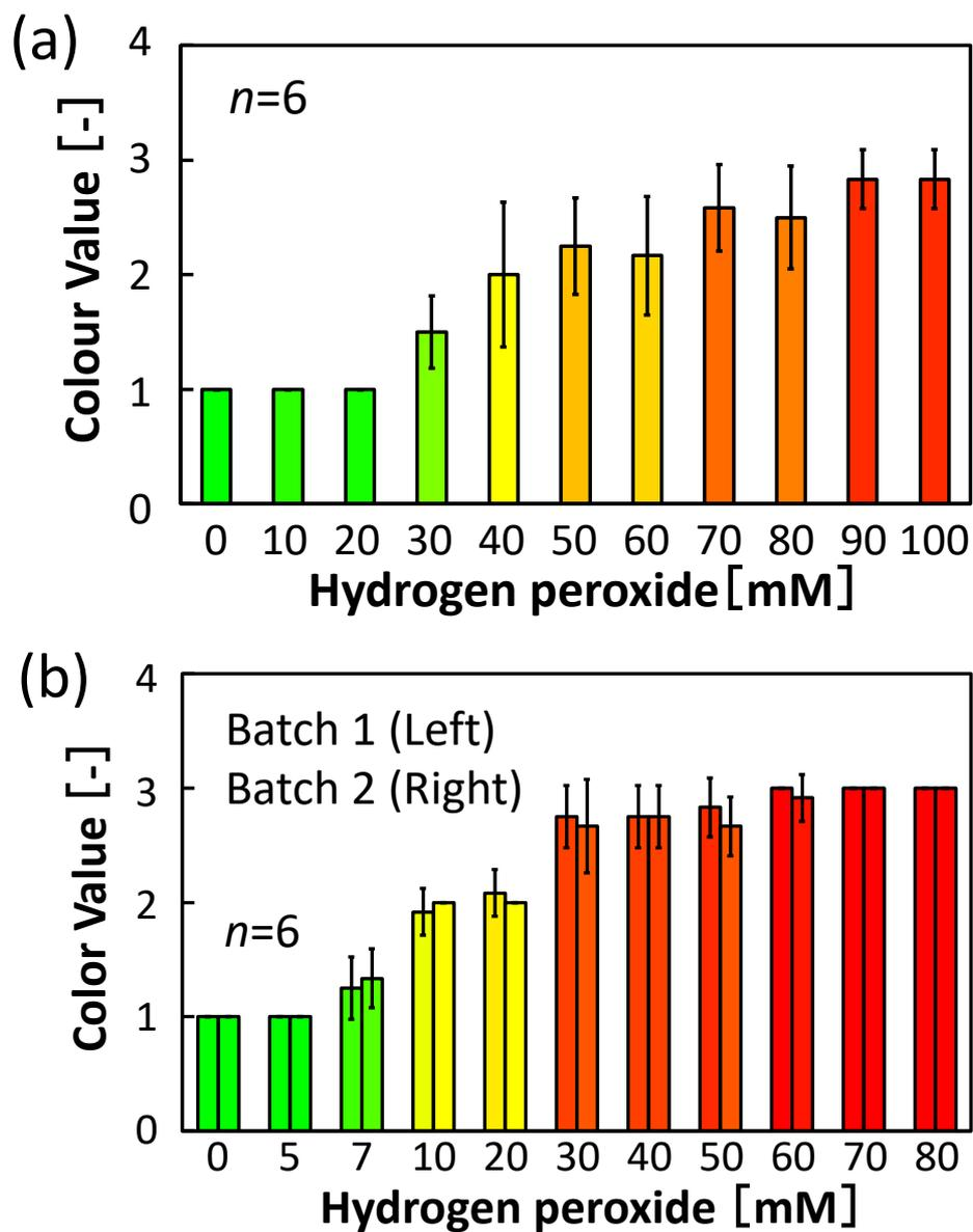
**Fig. S7** : Results of traffic light assay for  $H_2O_2$  detection using (a) Device 1, and (b) Device 2a demonstrating the reproducibility between two batches of devices independently fabricated within approximately 8 months. Error bars represent mean values  $\pm 1 \sigma$  for 6 individually fabricated  $\mu$ PADs.
