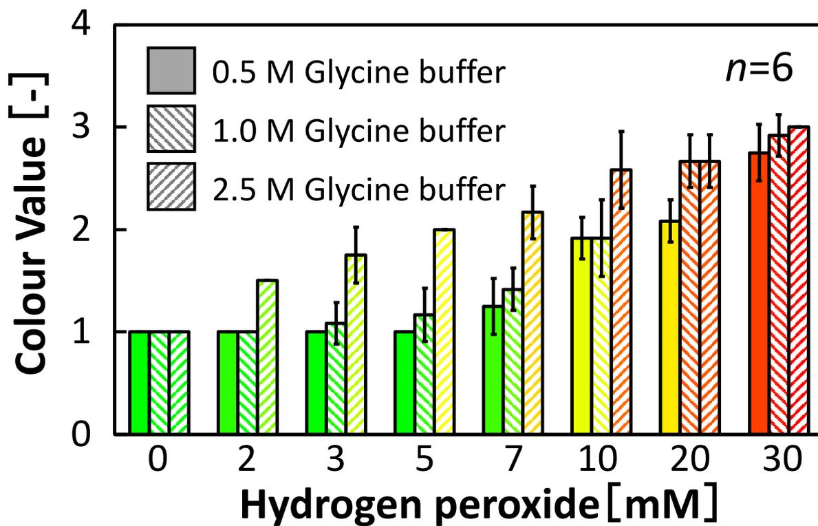
**Fig. S12** : Results of traffic light assay for H<sub>2</sub>O<sub>2</sub> detection demonstrating changes of the concentration threshold for displaying traffic light colours by increasing the concentration of the glycine buffer (pH 9.0) pre-deposited on the device (Device 2); error bars represent mean values  $\pm 1\sigma$  ( $n = 6$ ).
