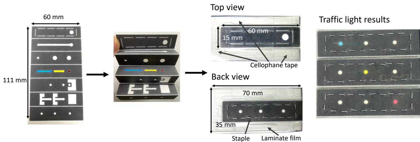
**Fig. S4** : Traffic light type  $\mu$ PAD assembly method (shown on the example of Device 2) and photographs of device backsides showing the traffic light signal (green, yellow or red) after the application of samples of various  $\text{H}_2\text{O}_2$  concentrations.
