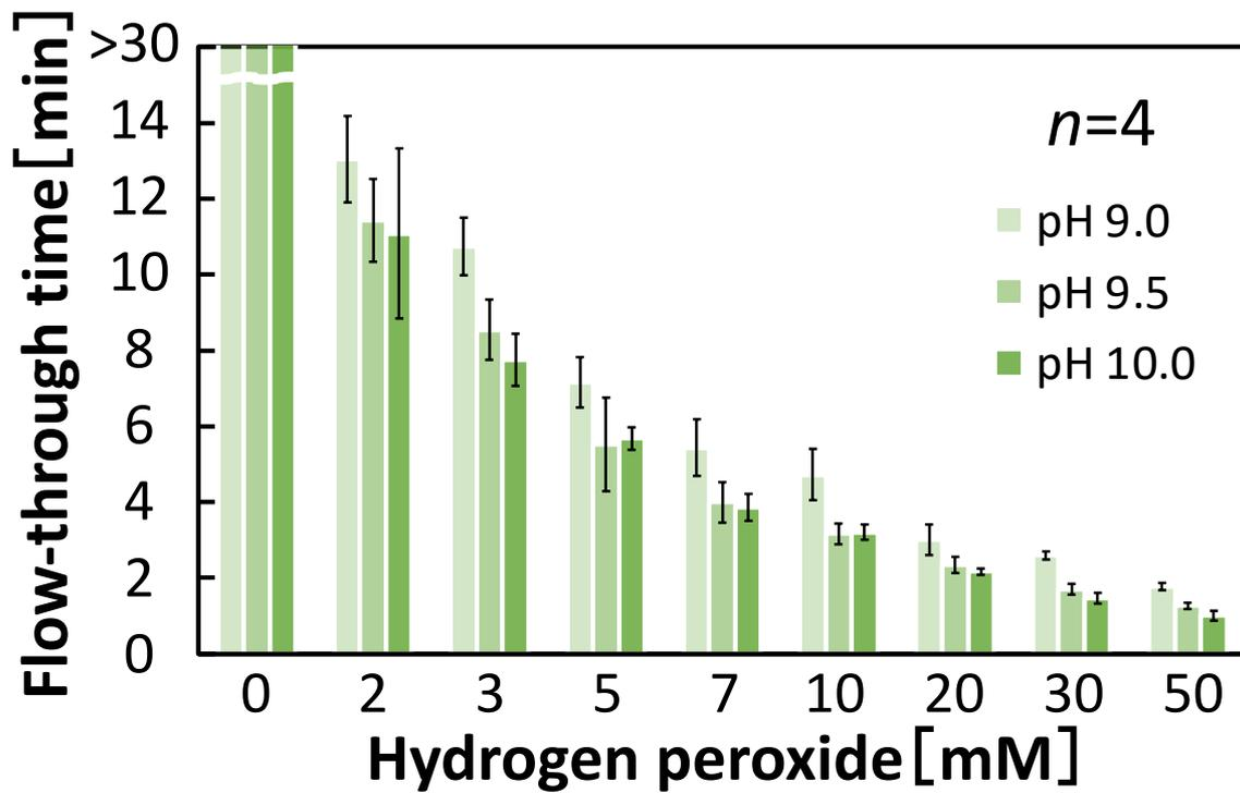
**Fig. S11** : Measurement of H<sub>2</sub>O<sub>2</sub> concentration-dependent flow-through times at different pH values (pH 9.0, 9.5, 10.0) using model Devices c-e (Fig. S2); error bars represent mean values  $\pm 1\sigma$  ( $n = 4$ ).
