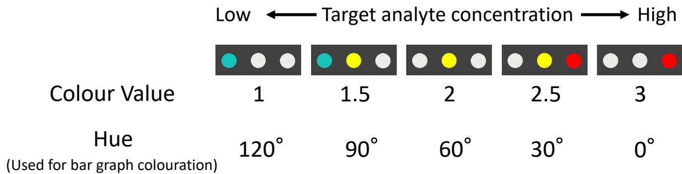
**Fig. S5** : Schematic illustration of the colour evaluation method to convert the traffic light colours into color values. The hue is used to support the visualization of quantitative results at a certain analyte concentration.
