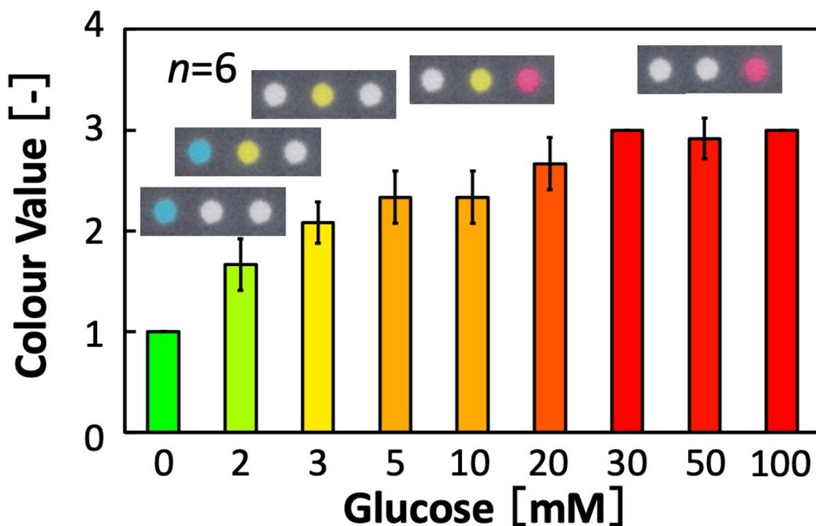
**Fig. S14** : Results of traffic light colour glucose assay from aqueous samples reacted with GOx off-device: (a) Device 2a and (b) Device 2b; error bars represent mean values  $\pm 1\sigma$  ( $n = 6$ ); insets show the actually observed traffic light signal for each respective analyte concentration (note: images of colored spots are cut and pasted next to each other in magnified form; refer to Fig. S4 for an example of an actual size image).
