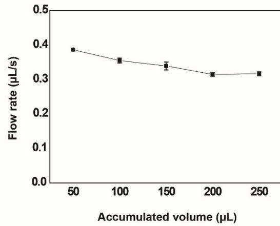
Figure S8: Plot of average flow rate as a function of sample volume measured during sample loading in P-CLIP experiments for solutions of sample and preprocessing reagents. Error bars represent  $\pm 1$  std. dev. from  $n = 5$  replicates in each condition.
