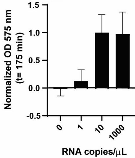
Figure S5: Optimized extraction conditions for detection limit using the Genesig Easy® kit. Plot showing normalized cell-free expression assay results implemented with the optimized ratio of Carrier RNA solution: Sample solution volume (0.25) using the manual workflow, which reduced detection limits to 1 copy/μL trigger RNA. Error bars represent 1 std. dev. from  $n = 3$  replicates in each condition.
