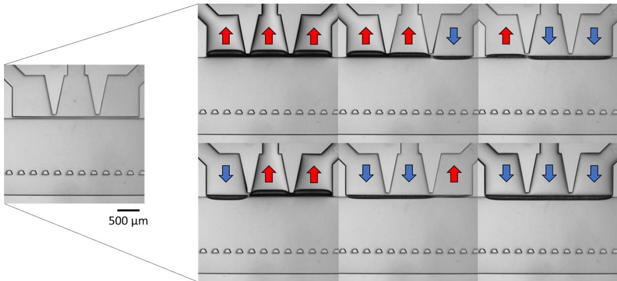
**Supplementary Figure 1:** Top view of the cartilage-on-chip system without any hydrogel matrix in the cell culture chamber. Deformation of the 50 µm thick PDMS membrane is achieved by applying positive (blue arrow) and/or negative (red arrow) pressure in the three individual actuation chambers generating a multi-directional mechanical stimulation pattern.
