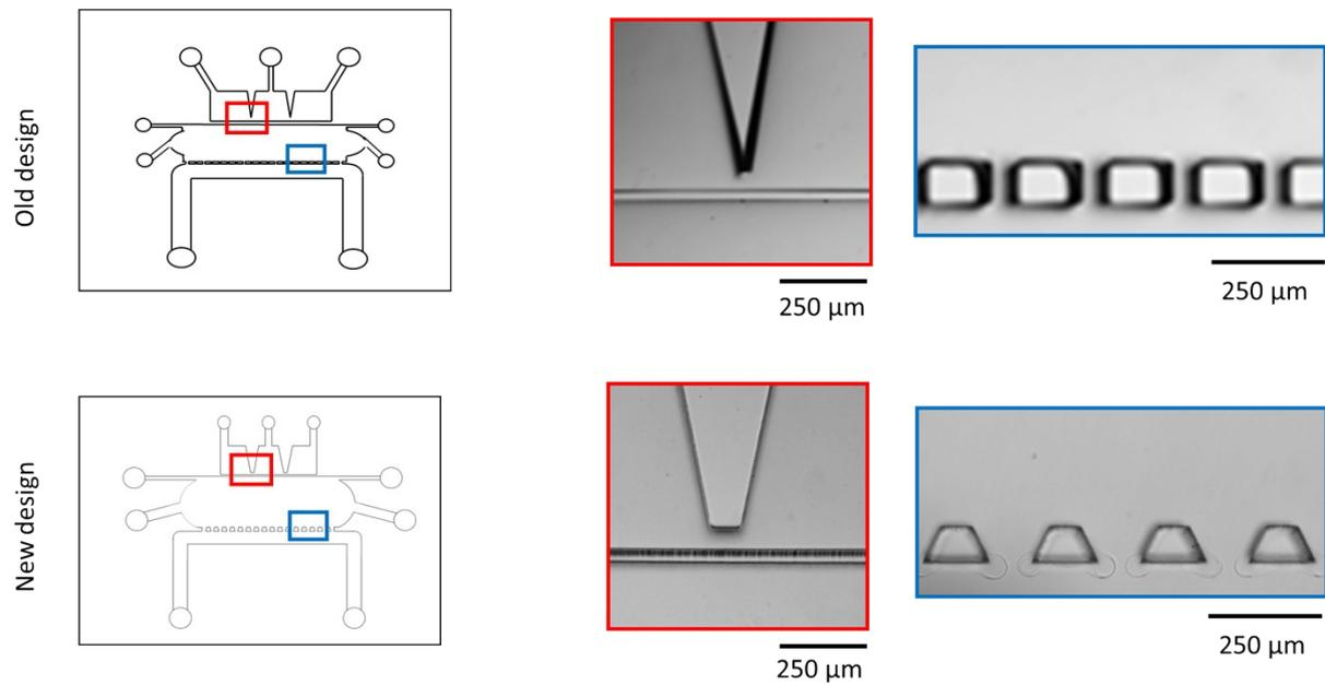
**Supplementary Figure 2:** *From left to right:* schematic representation of the top view of the old and new cartilage-on-chip devices, highlighting the applied modifications to the mechanical actuation (red square) and the pillars that separate the cell-hydrogel chamber from the perfusion (blue square). The aspect ratio of the membrane is increased as well, which is not depicted on this top view of the system.
