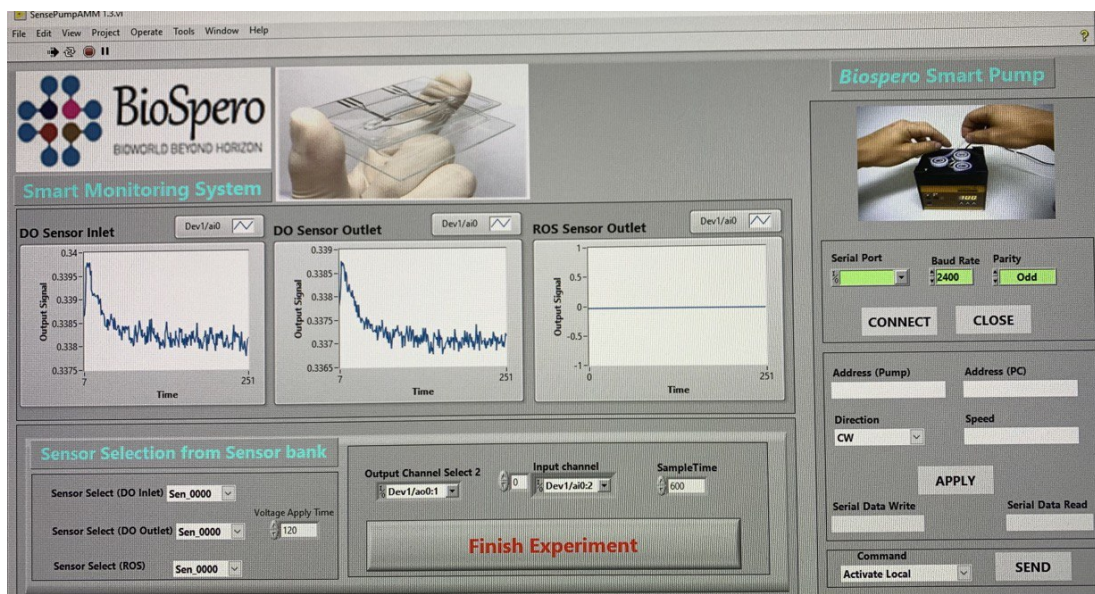
Figure S5. A snapshot of the data acquisition software showing the data for epithelium side DO sensors connected to the system. The change in output signal is because of the two different locations of DO sensors which shows the consumption of dissolved oxygen by Caco-2 epithelium in real time.
