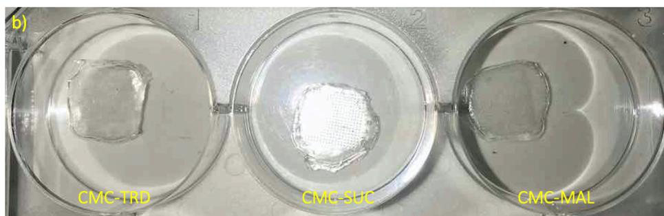
Figure S9 – Photos showing microneedle arrays after 6 months at 4°C
