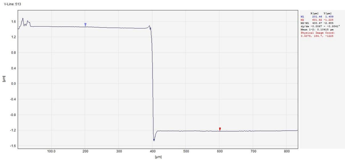
Figure F1 - Profile of the polymer film thickness on glass using white light profilometry.
