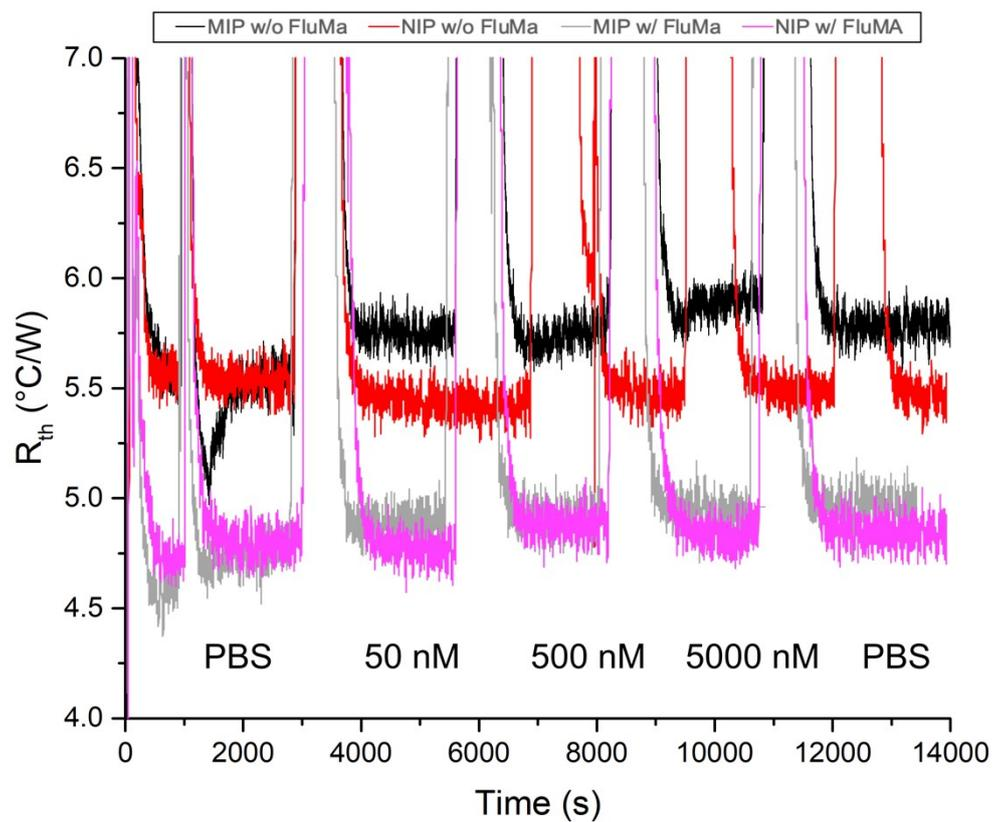
Figure G1 - Thermal resistance measurements for imprinted and non-imprinted polymer films with three layers, with injections of PBS containing increasing concentrations of nafcillin.
