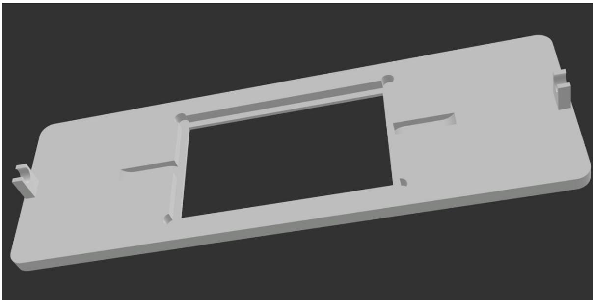
Figure C1 - 3D render of custom designed flow cell holder for microscope analysis.
