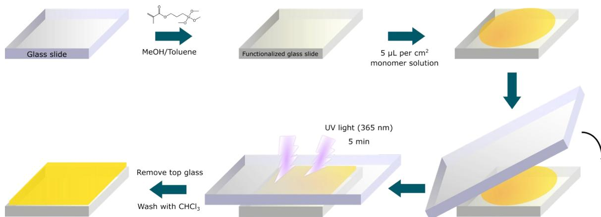
Figure B1 - Schematic of protocol for the formation of imprinted polymer films on glass substrate.
