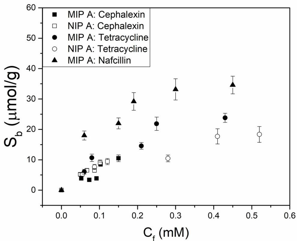
Figure E1 - Batch rebinding measurements using UV-vis spectroscopy for a nafcillin-imprinted polymer (MIP A) using solutions containing nafcillin, cephalexin and tetracycline in PBS.
