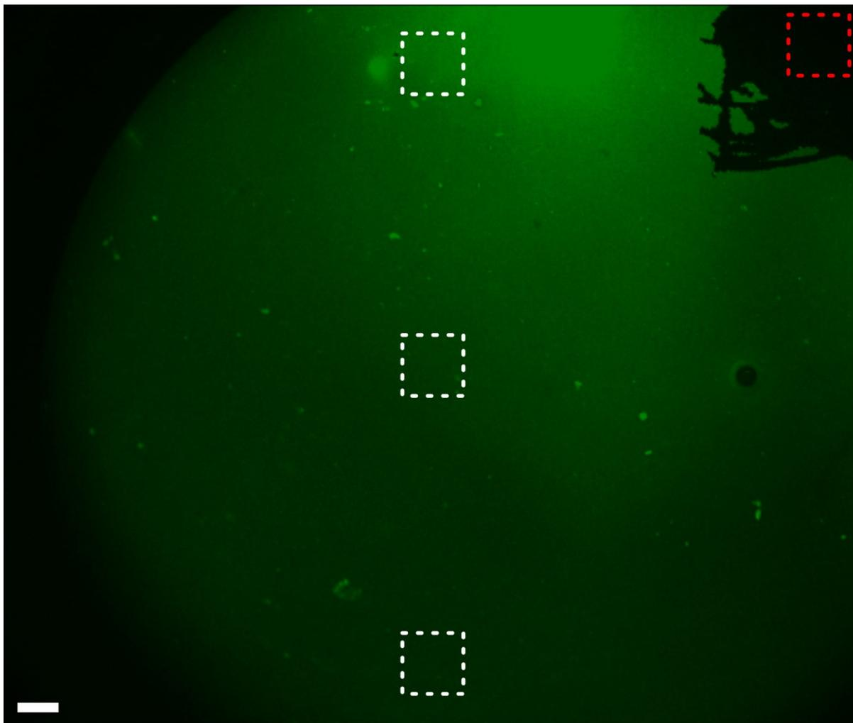
Figure D1 - Fluorescent micrograph of non-imprinted polymer film, showing regions of analysis (white) and background subtraction (red). [scale bar = 200  $\mu\text{m}$ ]
