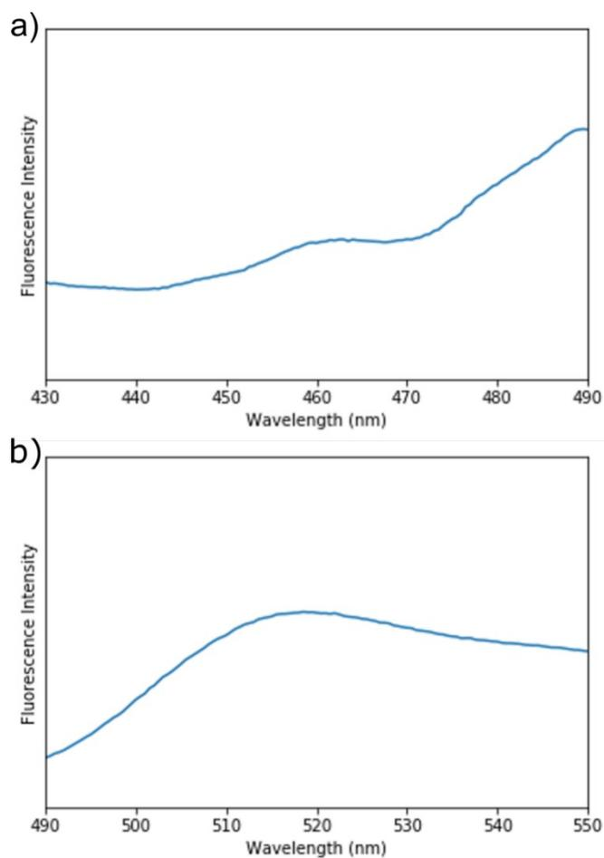
Figure H1 - Fluorescence spectra for FluMa-containing polymer film on glass in PBS, where a) is the excitation spectrum with  $\lambda_{em} = 515$  nm, and b) is the excitation spectrum with  $\lambda_{ex} = 460$  nm.
