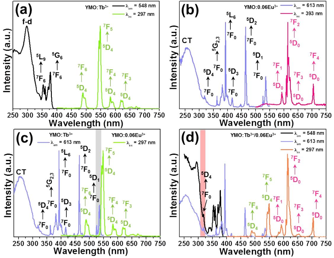
**Figure S3.** Excitation and emission spectra of (a) YMO:Tb<sup>3+</sup> and (b) YMO:0.06Eu<sup>3+</sup> NTE microparticles. (c) Excitation spectrum of YMO:0.06Eu<sup>3+</sup> NTE microparticles and emission spectrum of YMO:Tb<sup>3+</sup> NTE microparticles. (d) Excitation and emission spectra of YMO:Tb<sup>3+</sup>/0.06Eu<sup>3+</sup> NTE microparticles.
