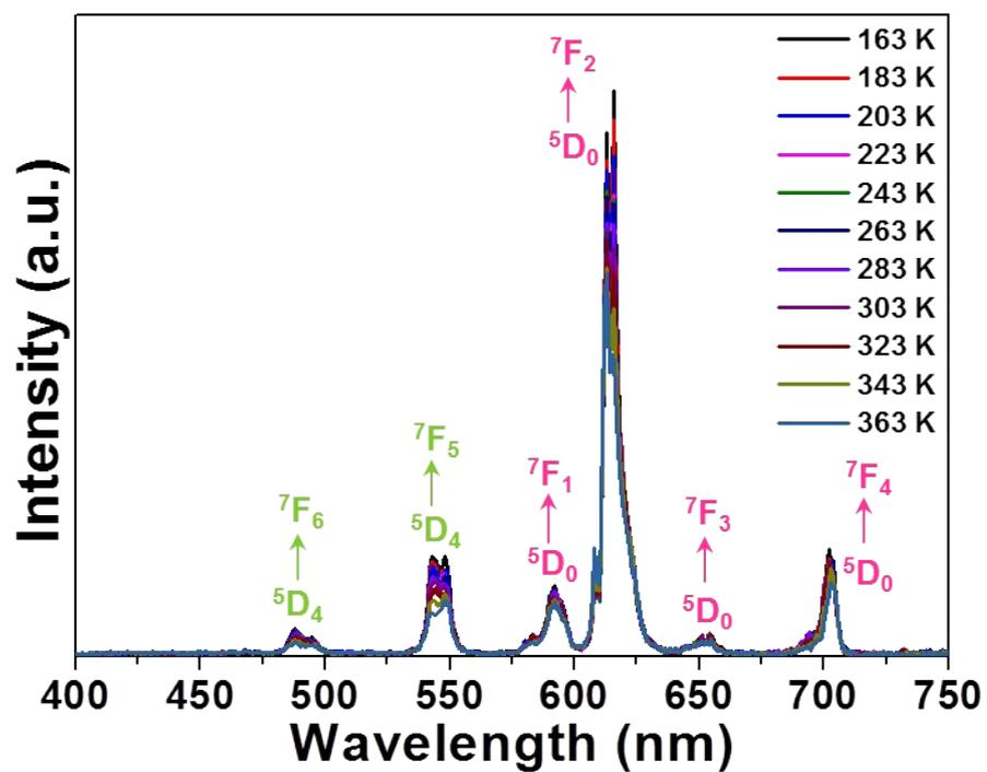
**Figure S8.** Emission spectra of the YMO:Tb<sup>3+</sup>/0.10Eu<sup>3+</sup> NTE microparticles excited by 297 nm as a function of temperature.
