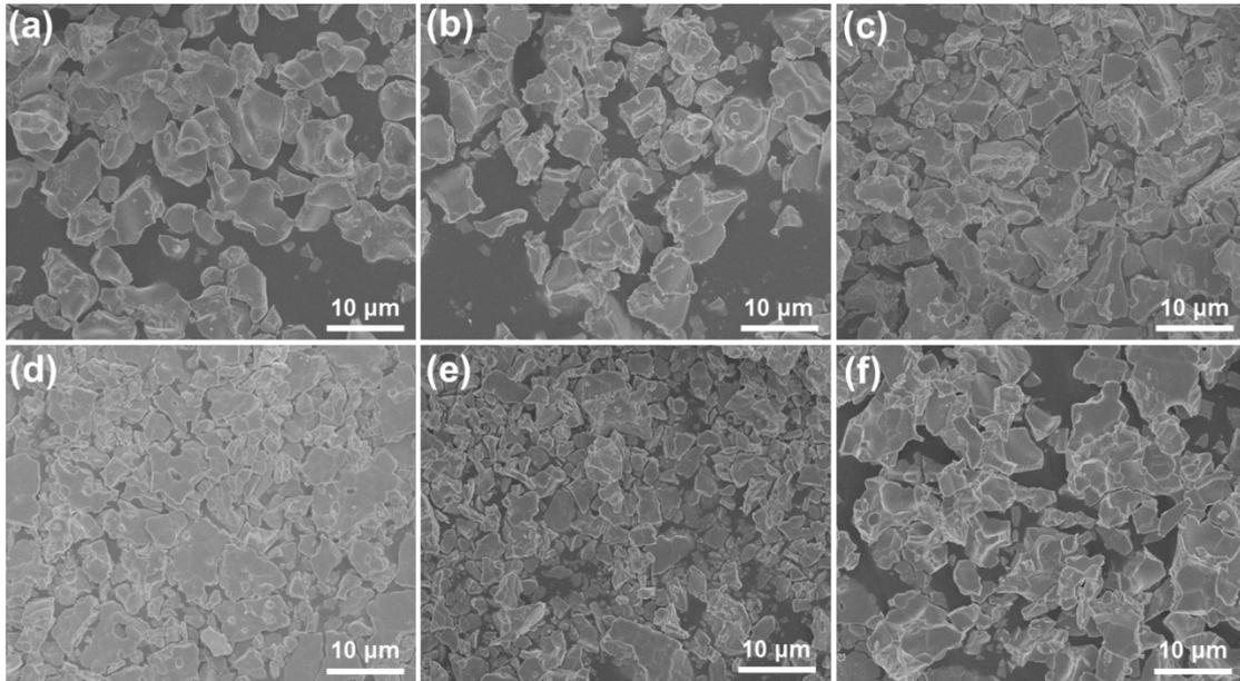
**Figure S1.** (a) FE-SEM image of YMO:0.06Eu<sup>3+</sup> NTE microparticles. FE-SEM images of YMO:Tb<sup>3+</sup>/2xEu<sup>3+</sup> NTE microparticles with different doping concentration of (b)  $x = 0$ , (c)  $x = 0.01$ , (d)  $x = 0.05$ , (e)  $x = 0.07$  and (f)  $x = 0.09$ .
