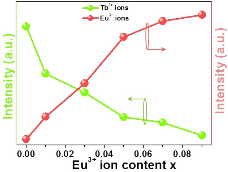
**Figure S4.** Emission intensities of Tb<sup>3+</sup> and Eu<sup>3+</sup> ions in YMO:Tb<sup>3+</sup>/2xEu<sup>3+</sup> NTE microparticles as a function of doping concentration.
