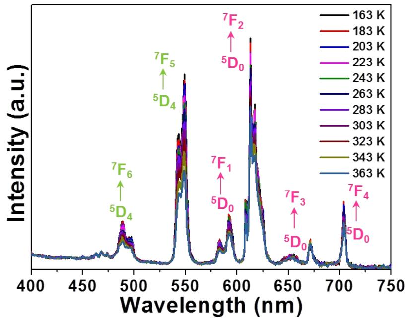
**Figure S9.** Emission spectra of the YMO:Tb<sup>3+</sup>/0.06Eu<sup>3+</sup> NTE microparticles excited by 378 nm as a function of temperature.
