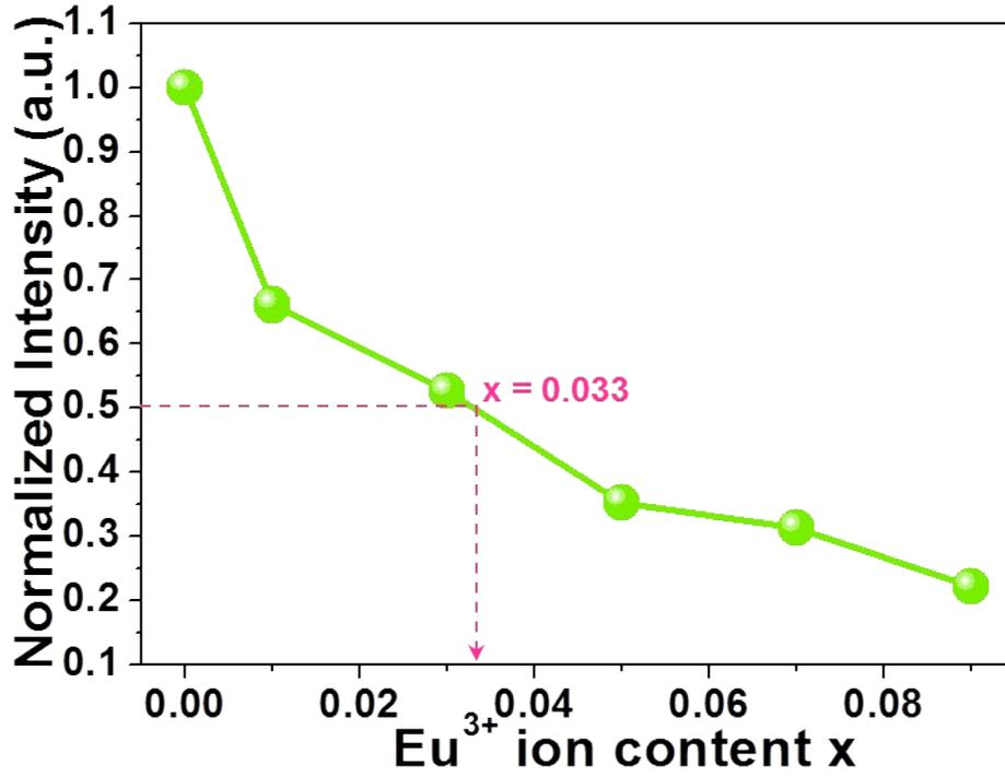
**Figure S5.** Normalized emission intensity of Tb<sup>3+</sup> ions in YMO:Tb<sup>3+</sup>/2xEu<sup>3+</sup> NTE microparticles as a function of Eu<sup>3+</sup> ion content.
