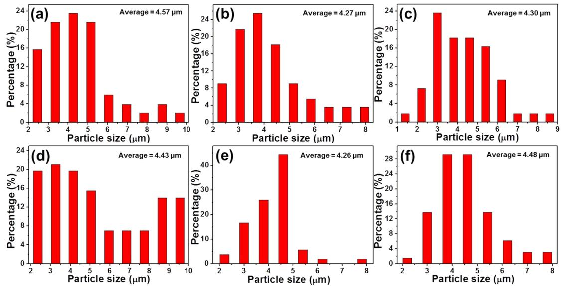
**Figure S2.** (a) Particle size distribution of YMO:0.06Eu<sup>3+</sup> NTE microparticles. Particle size distribution of YMO:Tb<sup>3+</sup>/2xEu<sup>3+</sup> NTE microparticles with different doping concentration of (b)  $x = 0$ , (c)  $x = 0.01$ , (d)  $x = 0.05$ , (e)  $x = 0.07$  and (f)  $x = 0.09$ .
