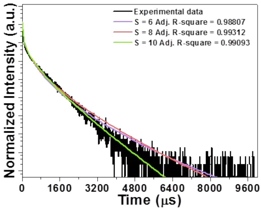
**Figure S6.** Fitted decay curve of YMO:Tb<sup>3+</sup>/0.18Eu<sup>3+</sup> NTE microparticles monitored at 378 nm by using the I-H model
