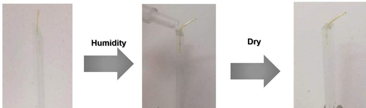
**Figure S10.** Time-lapse images of the bending response of the H-bonded network (Thickness =50  $\mu\text{m}$ ) to water vapor flow and remained in the bent state after switching to dry condition for three hours.
