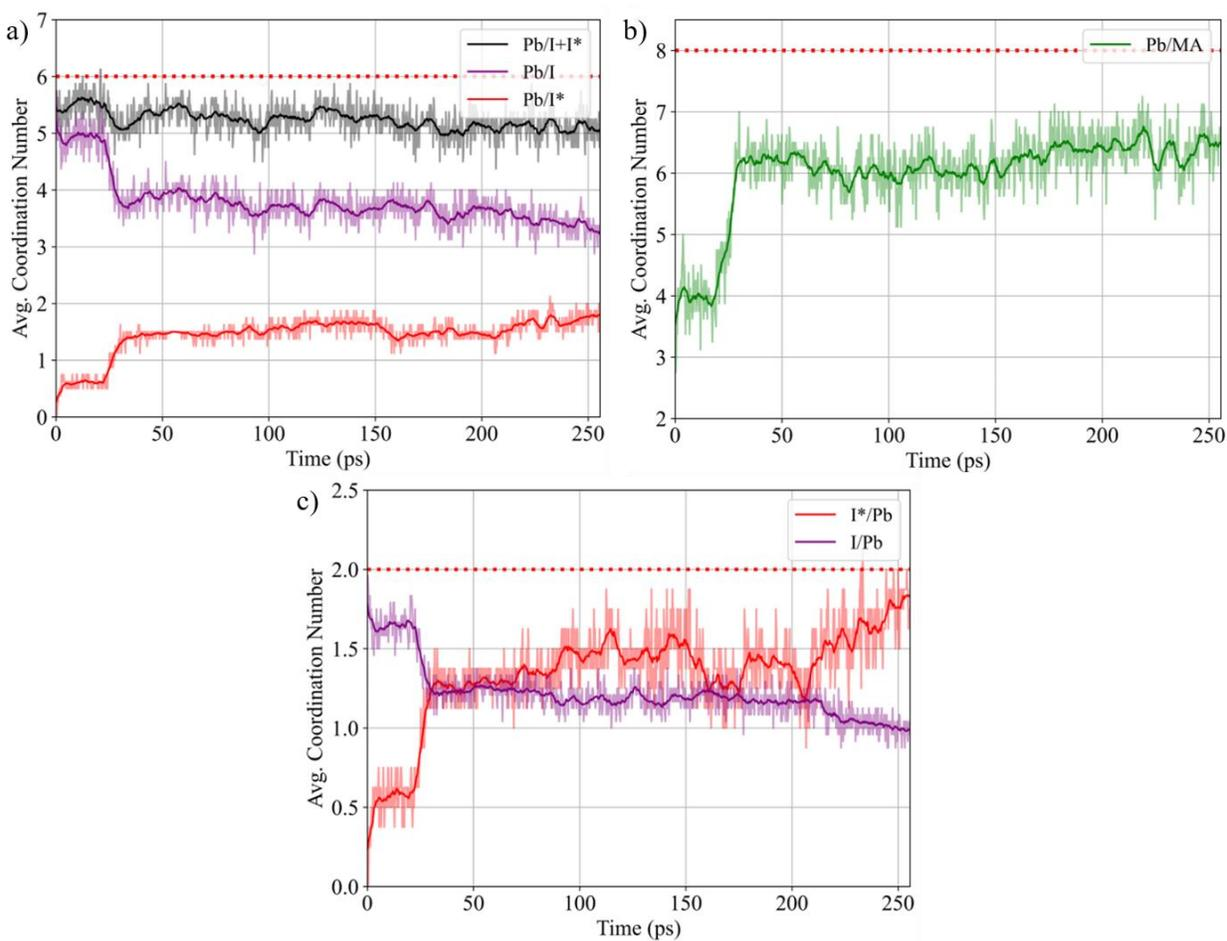
**Figure S6.** Time evolution of the average coordination number of (a) lead with iodide coming from  $PbI_2$  ( $Pb/I$ ) and iodide coming from MAI ( $Pb/I^*$ ), and the sum of both contributions ( $Pb/I+I^*$ ); (b)  $Pb/MA$  coordination number; (c)  $I^*/Pb$  and  $I/Pb$  coordination number. The solid lines show a moving average with time window of 5 ps. The dotted red line highlights the expected coordination number of bulk  $MAPbI_3$ .
