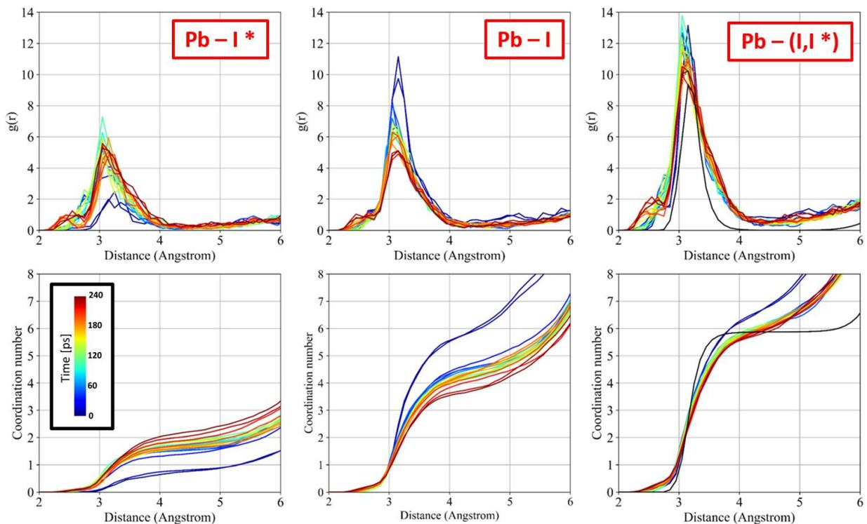
**Figure S9.** Time evolution of the (top) radial distribution function  $g(r)$  and (bottom) coordination number of (left) Pb-I\*, (mid) Pb-I, and (right) the sum of both. The colors capture the time information: blue = initial distribution, red = final distribution. In the right subplots, the black line shows the expected  $g(r)$  and coordination number for the orthorhombic phase of MAPbI<sub>3</sub>.
