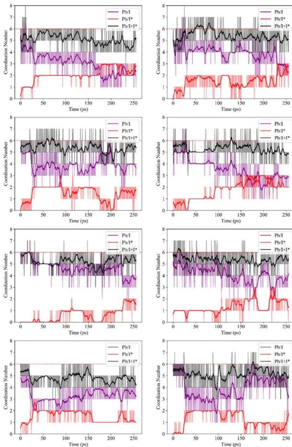
**Figure S2.** Time evolution of the coordination number of each lead ion with iodine coming from  $\text{PbI}_2$  ( $\text{Pb/I}$ ) and iodine coming from MAI ( $\text{Pb/I}^*$ ), and the sum of both contributions ( $\text{Pb/I+I}^*$ ).
