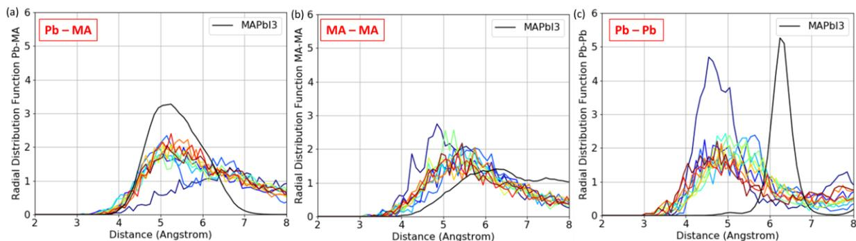
**Figure S10.** Radial distribution functions (RDF) for (a) Pb-MA, (b) MA-MA, (c) Pb-Pb. Nitrogen has been used as a reference for the methylammonium cation. The black line shows the expected cumulative RDF for the perovskite phase of MAPbI<sub>3</sub>. The colors capture the time information of the RDF: time increases from blue to red. All curves show averages across 100 trajectory snapshots (~25 ps).
