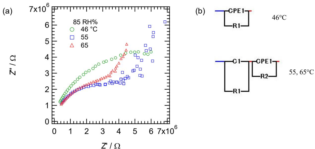
**Fig. S2** (a) Nyquist plot for **1CT-18C6-I** at 46, 55, and 65 °C under 85 RH% humidity and (b) equivalent circuit models for the fitting to data of 46 °C (top) and 55 and 65 °C (bottom).
