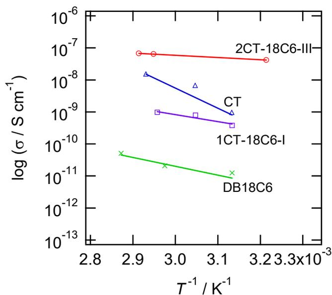
**Fig. S6** Arrhenius plot of proton conductivity under 85 RH%.
