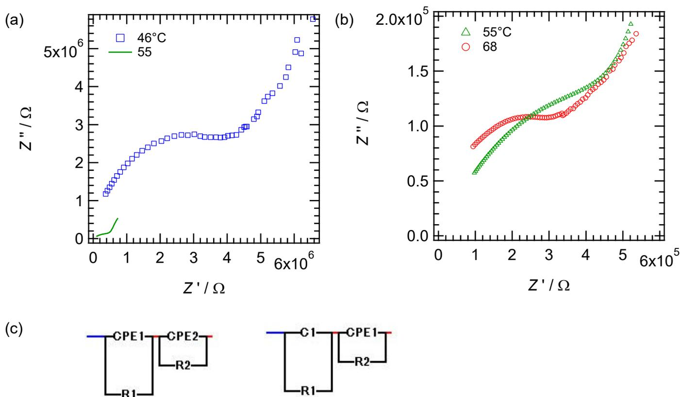
**Fig. S3** (a) Nyquist plot for CT at 46, 55, and 68 °C under 85 RH% humidity and (b) equivalent circuit models for the fitting to data of 46 °C (top) and 55 and 68 °C (bottom).
