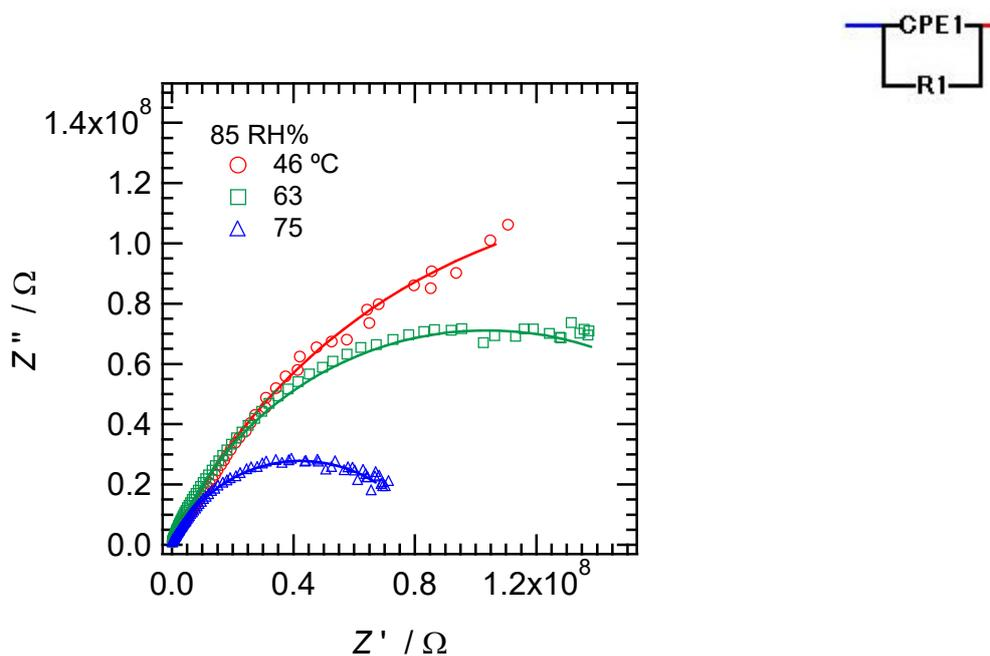
**Fig. S4** (a) Nyquist plot for DB18C6 at 46, 63, and 75 °C under 85 RH% humidity and (b) equivalent circuit models for the fitting to data.
