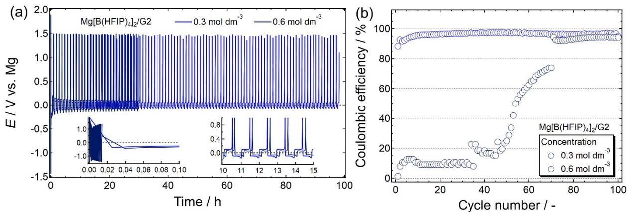
**Figure S11.** (a) Galvanostatic magnesium deposition/dissolution cycling profiles and (b) corresponding Coulombic efficiency in  $0.3$  and  $0.6 \text{ mol dm}^{-3}$   $Mg[B(HFIP)_4]_2/G2$ . The  $0.6 \text{ mol dm}^{-3}$  solution required over 60 times of pre-cycling to complete the conditioning of the electrolyte and/or [electrolyte | anode] interface.
