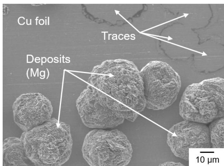
**Figure S2.** SEM image of Cu working electrode after galvanostatic polarization at  $1 \text{ mA cm}^{-2}$  for 1 h in  $0.3 \text{ mol dm}^{-3} \text{ Mg}[\text{Al}(\text{HFIP})_4]_2/\text{G2}$  at  $30 \text{ }^\circ\text{C}$ .
