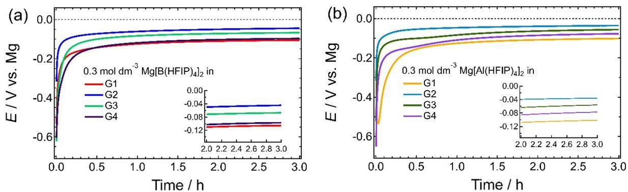
**Figure S6.** Voltage profiles of galvanostatic polarization in (a)  $0.3 \text{ mol dm}^{-3} \text{Mg}[\text{B}(\text{HFIP})_4]_2/\text{G}n$  and (b)  $0.3 \text{ mol dm}^{-3} \text{Mg}[\text{Al}(\text{HFIP})_4]_2/\text{G}n$  ( $n = 1-4$ ) recorded on carbon fiber electrodes at  $1 \text{ mA cm}^{-2}$  at 30 °C. Insets display the magnified profiles of the steady state.
