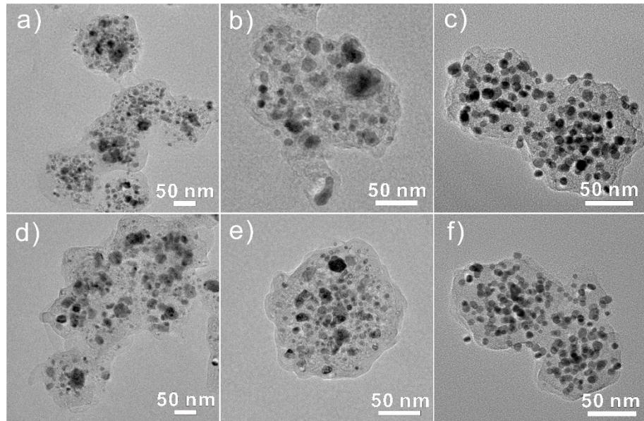
**Fig. S8** TEM images of Pt-CoZn@NC-800-10% (a) before and (d) after ADT, Pt-Co@NC-800-10% (b) before and (e) after ADT, and Pt-Zn@NC-800-10% (c) before and (f) after ADT.
