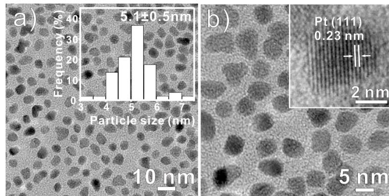
**Fig. S1** (a-b) TEM images of PVP capped Pt NPs. The inset in (a) shows the particle size distribution, and the inset in (b) shows the interplanar spacing of Pt NPs.
