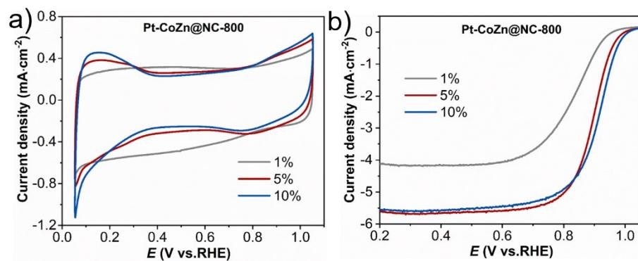
**Fig. S9** (a) CV curves and (b) polarization curves of Pt-CoZn@NC-800 catalysts with different Pt loading amounts.
