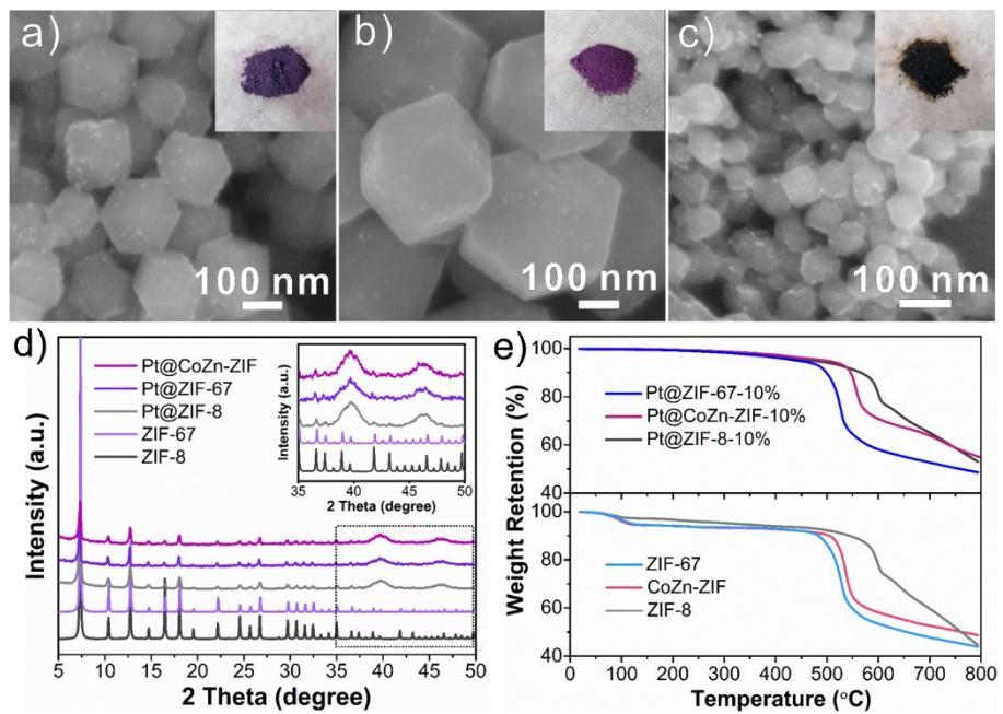
**Fig. S2** SEM image and photographs of (a) Pt@CoZn-ZIF, (b) Pt@ZIF-67, and (c) Pt@ZIF-8. (d) Powder XRD patterns of precursors and ZIFs. The inset shows detail patterns from 35 to 50 degree. (e) TGA curves of precursors and ZIFs. Here the content of Pt NPs in every precursors is 10 wt<sub>Pt</sub>%.
