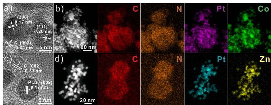
**Fig. S4** (a) HRTEM image and (b) HAADF-STEM image with corresponding element mappings of Pt-Co@NC-800-10% catalyst. (c) HRTEM image and (d) HAADF-STEM image with the corresponding element mappings of Pt-Zn@NC-800-10% catalyst.
