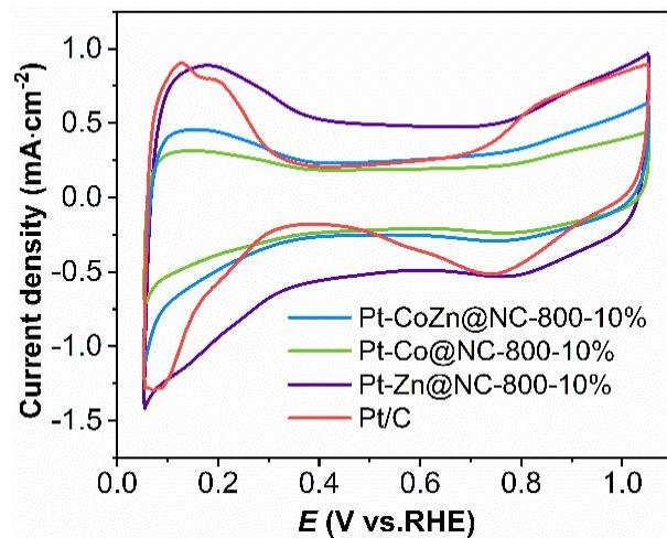
**Fig. S6** CV curves of three catalysts in a N<sub>2</sub>-saturated 0.1 M HClO<sub>4</sub> solution with scan rate of 50 mV·s<sup>-1</sup>.
