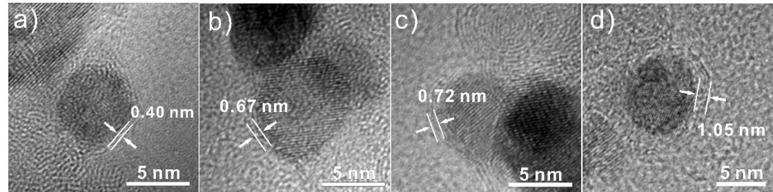
**Fig. S3** (a-d) HRTEM images of alloy NPs embedded in the carbon matrix of Pt-CoZn@NC-800-10%.
