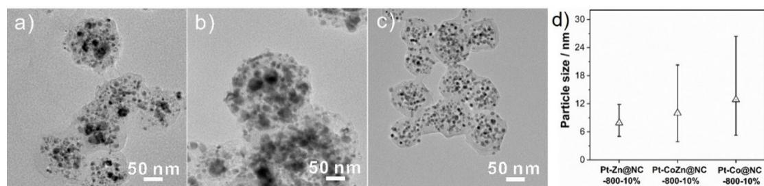
**Fig. S5** TEM images of (a) Pt-CoZn@NC-800-10%, (b) Pt-Co@NC-800-10%, and (c) Pt-Zn@NC-800-10%. (d) The size distribution of alloy nanoparticles of three samples.
