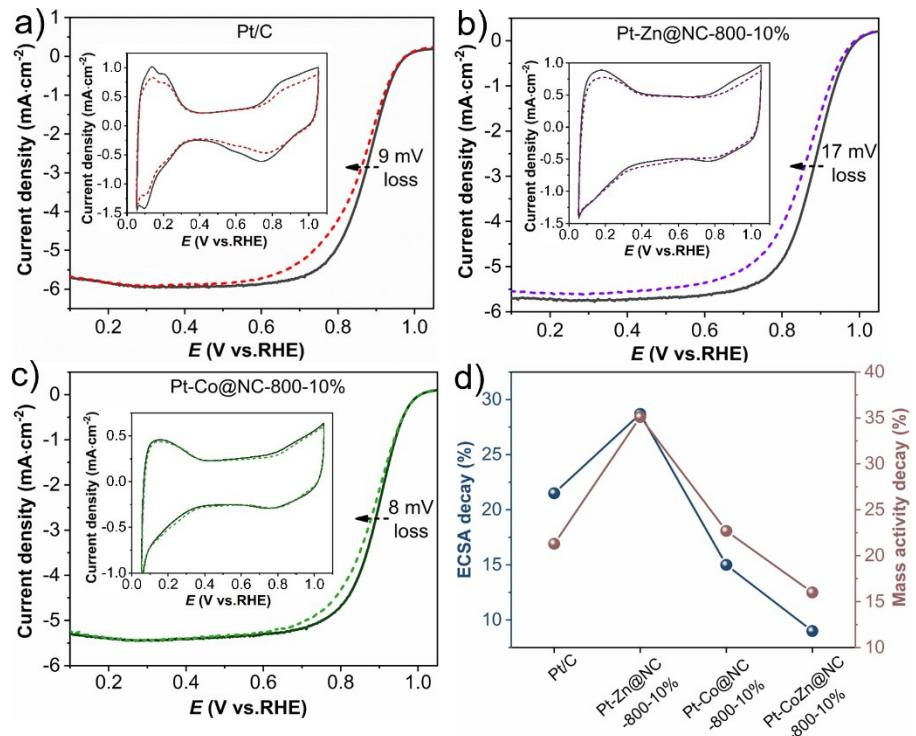
**Fig. S7** ORR polarization curves of (a) the commercial Pt/C, (b) Pt-Zn@NC-800-10%, and (c) Pt-Co@NC-800-10% catalysts before and after 5,000 cycles in ADT. The insets show the change of CV results. (d) The decay of mass activity and ECSA for different catalysts during ADT.
