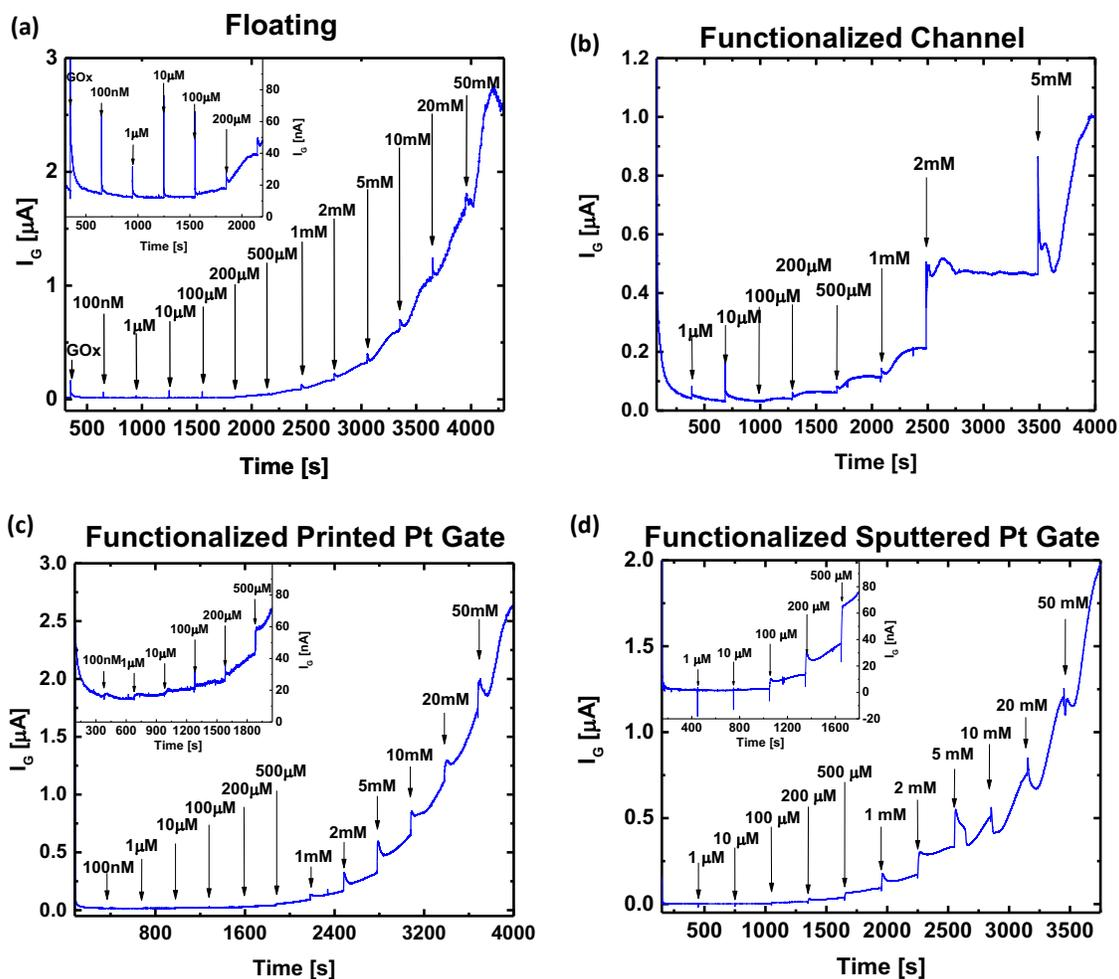
Figure S2. The corresponding  $I_G$  response of the four OECT functionalization configurations as shown in Figure 3. (a) Unfunctionalized OECT with floating GOx. (b) OECT with functionalized channel. (c) OECT with functionalized printed Pt gate. (d) OECT with functionalized sputtered Pt gate. At higher glucose concentrations,  $I_G$  keeps increasing due to the limited GOx amount for glucose molecule oxidation and limited Pt surface area for  $\text{H}_2\text{O}_2$  decomposition.
