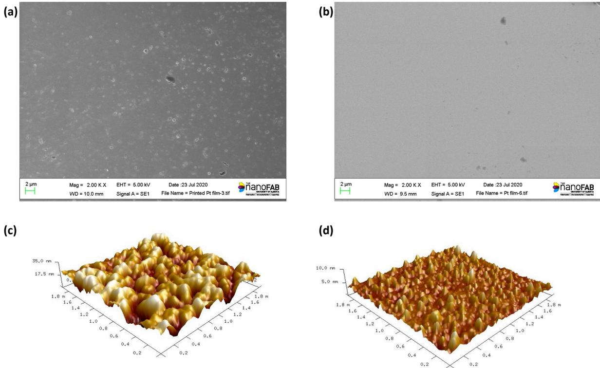
Figure S3. Surface roughness comparison of printed and sputtered Pt films. (a) Scanning electron microscopic (SEM) image of printed Pt film. (b) SEM image of Pt thin film deposited by magnetron sputter system. (c) Atomic force microscopic (AFM) image of printed Pt film. (d) AFM image of sputtered Pt film. The printed nanoparticle-based Pt film has higher surface RMS roughness ( $R_q$ ) of 13.8 nm as compared to  $R_q = 0.852$  nm for the sputtered Pt film.
