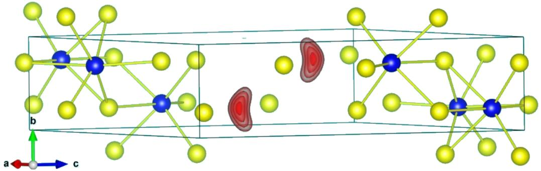
**Figure S1.** 3D isosurface of the Fourier difference maps showing the bean-shaped electronic density of Tl after refinement of the Mo-S framework (isosurface levels at 20, 30, 40 and 50 e/Å<sup>3</sup> from light to dark red, Mo and S atoms are shown in blue and yellow, respectively).
