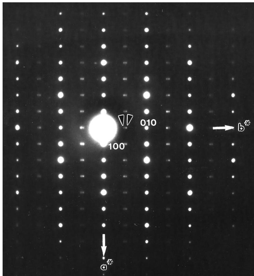
**Figure S3.** Electron diffraction images collected on crushed polycrystalline  $\text{Tl}_{0.6}\text{Mo}_3\text{S}_5$  in the  $ab$  plane. In addition to the main reflections, two rows of additional reflections (marked the black arrowheads) are observed, suggesting the presence of an incommensurate modulation running along the  $b$  axis.
