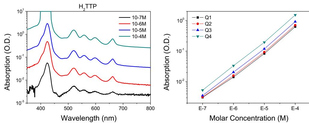
Figure S3 - Absorption spectra of H<sub>2</sub>TP porphyrin ranging from  $10^{-4}$  to  $10^{-7}$  M in THF and the linear behavior of the Q-bands with concentration.
