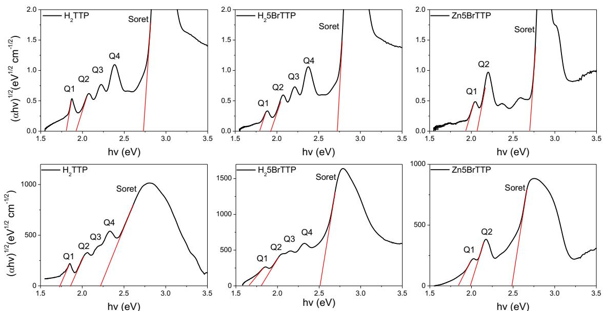
Figure S2 – Tauc plot analysis for UV-Vis spectra of H<sub>2</sub>TTP, H<sub>2</sub>5BrTTP and Zn5BrTTP in solution (first row) and thin film (second row).
