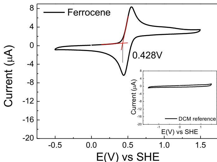
Figure S1 – The characteristic voltammogram of Ferrocene(Fc/Fc<sup>+</sup>) as reference sample. Two peaks of oxidation and reduction were observed at 0.548 V and 0.445 V, respectively. The potential obtained through the onset methodology is located at 0.428 V. The insert figure shows the solvent DCM voltammogram profile.
