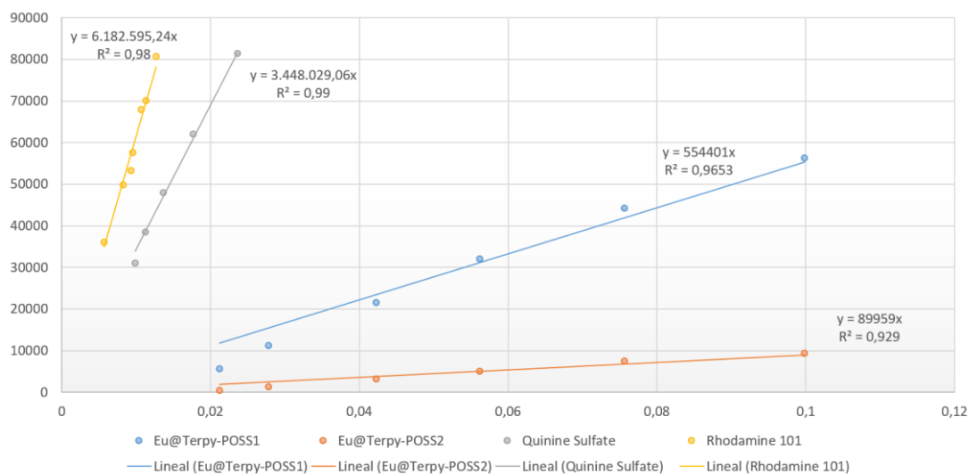
Figure S22. Quantum yield Ter-POSS@4Eu. The graph reports the fluorescence intensity (y) vs the absorption intensity at excitation wavelength (x).
