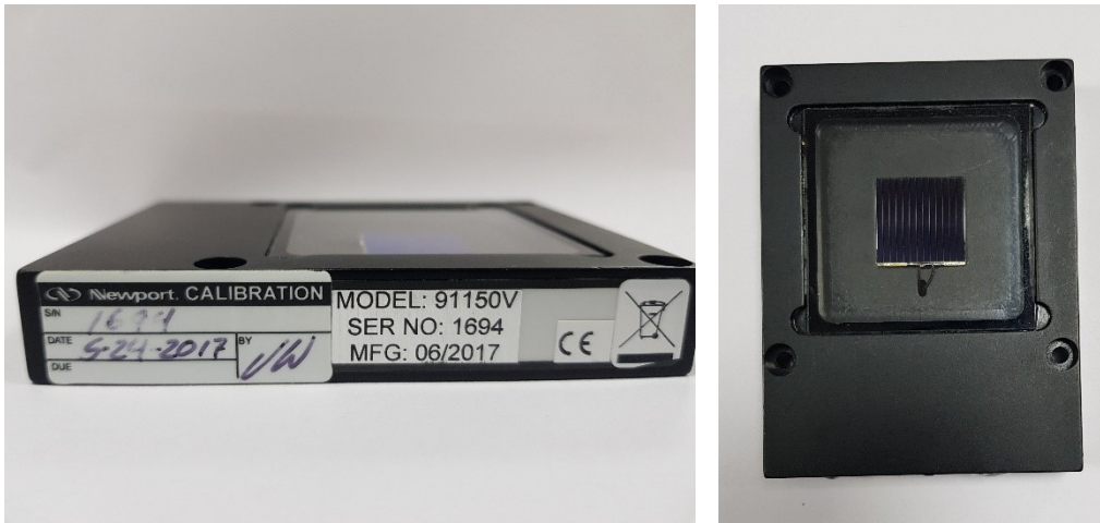
Figure S17. Standard silicon reference cell (Model: 91150V, S/N: 1694) calibrated by Newport.
