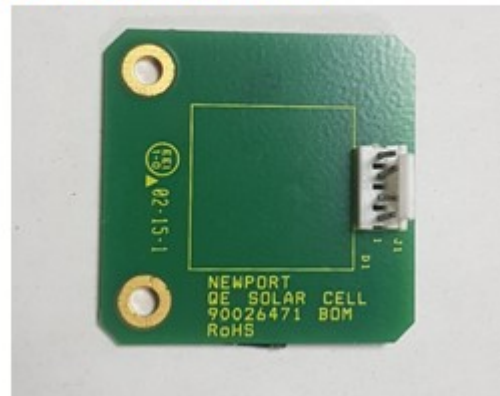
Figure S19. Detector and silicon reference cell for IPCE measurement.
