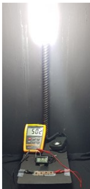
Figure S9. Image of self-powered temperature sensor with LCD display at 500 lux (Osram 14 W T2 cool day light fluorescent tube illumination) integrated with four serially connected DSCs fabricated with YK 8 sensitizer.
