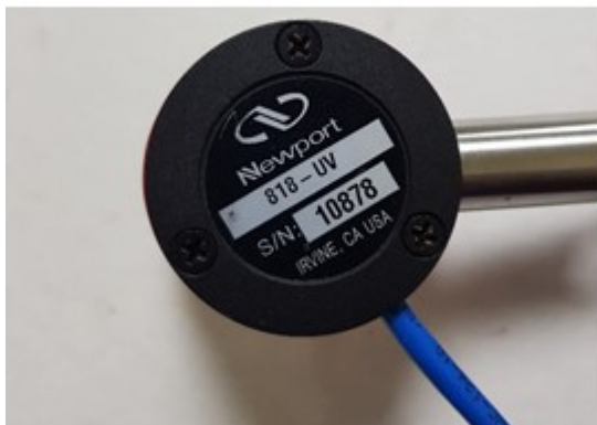
Figure S19. Detector and silicon reference cell for IPCE measurement.
