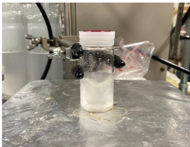
Fig. S1 The photograph of a convenient ball-milling method used in this work.
