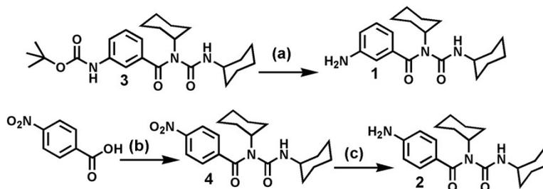
**ESI Figure S1.** The schematic representation for the synthesis of peptide mimetics **1** and **2**. Reagents and conditions: (a) TFA, DCM, 1h 95% (b) DCC, DCM, reflux, 5h, 75%, (c) (1:1) Fe, AcOH, Acetone-H<sub>2</sub>O, reflux 4h, 70%.
