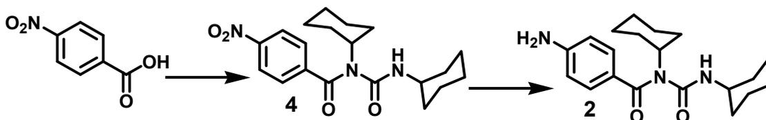
**Compound 4:** p-nitrobenzoic acid (1.67 g, 10 mmol) was dissolved in 60 mL of DCM at room temperature.  $\text{N,N}'$ -dicyclohexylcarbodiimide(DCC) (3.1 g, 15 mmol) and  $\text{Et}_3\text{N}$  (2 mL,
