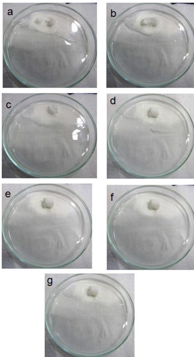
**ESI Figure S5.** The gel gets deformed towards strong mineral acid such as (a)  $\text{H}_2\text{SO}_4$  (b)  $\text{HNO}_3$ . The gel is sensitive to (c) acetic acid but not (d) formic acid. The gel is not responsive to (e)  $\text{NH}_3$ , (f) methylamine and (g) ethylamine.
