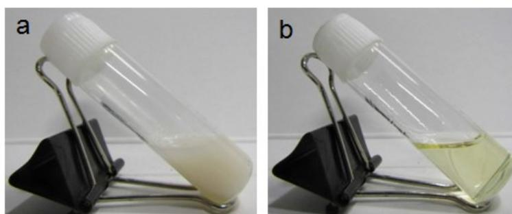
**ESI Figure S2.** The compound **1** forms white suspension in methylcyclohexane and clear solution in chloroform.
