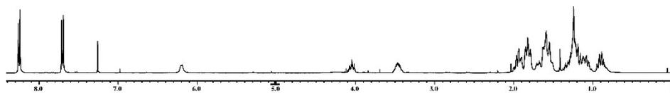
**Figure S10:**  $^1\text{H}$  NMR (400 MHz,  $\text{CDCl}_3$ ,  $\delta$  in ppm) spectra of compound 4.
