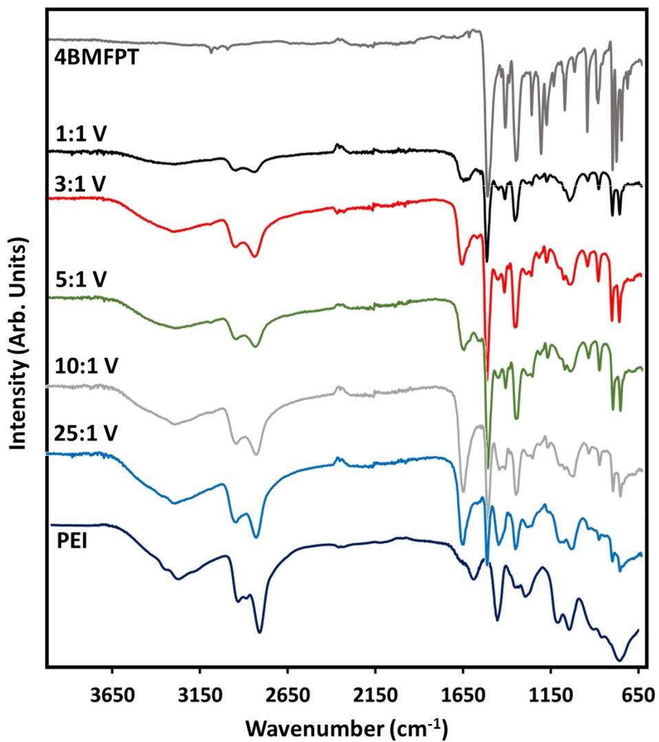
**Figure S3.** FTIR-ATR spectra of starting materials and PEI:4BMFPT cross-linked products.
