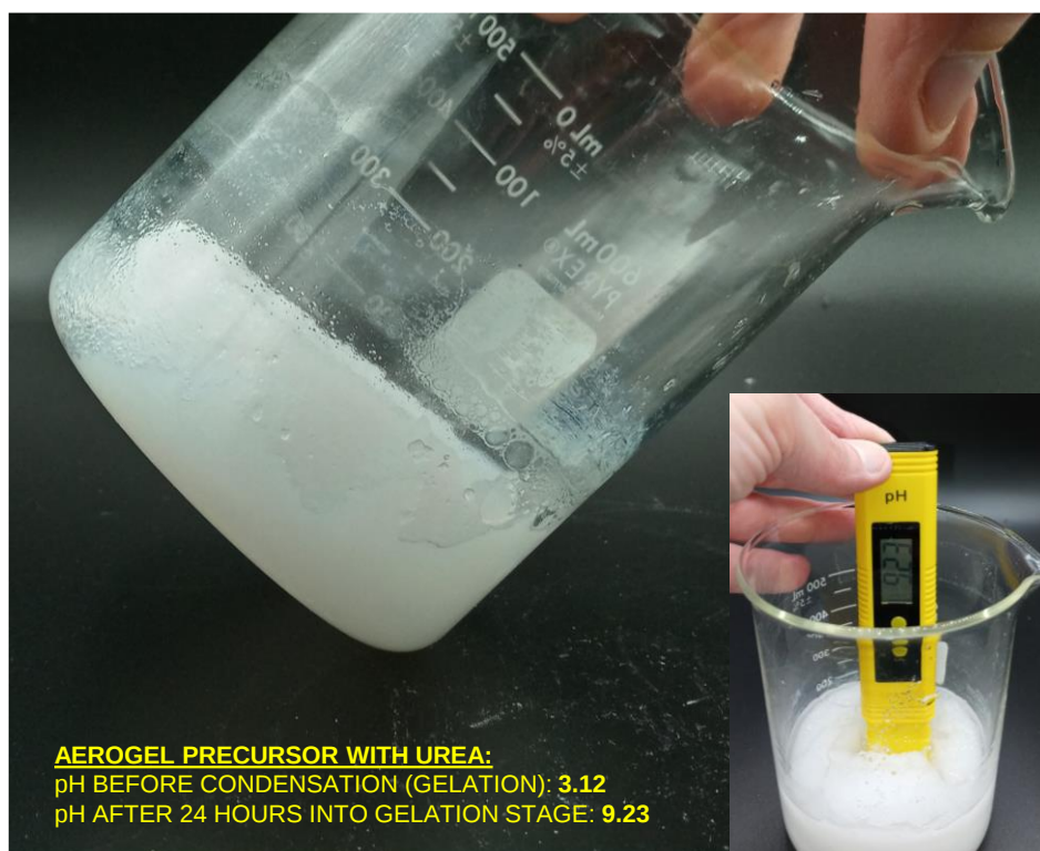
Figure S8. Optical image of aerogel precursor without (a) and with (b) urea after 24 hours into gelation stage. Inset images include pH measurement of the precursor.
