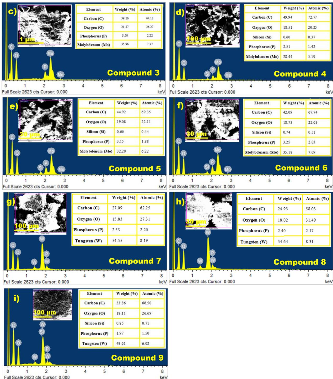
**Fig. S6.** a-i) FESEM-EDX for mesoporous compounds 1-9. The sample surface shows the presence of C, O, P (and/or Si) and Mo (or W) in the respective compounds. The weight and atomic percentages are summarized in tabular form.
