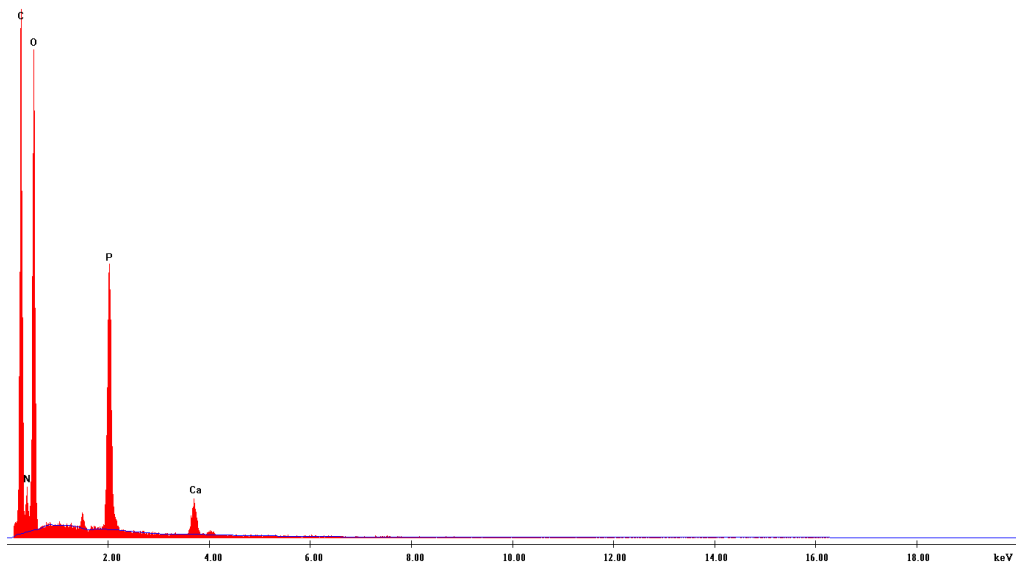
Figure S6.2.1. Energy dispersive spectra of ZOLE-Ca form I BPCC displaying the presence of atoms (carbon, nitrogen, oxygen and phosphorous) present in ZOLE and the metal (calcium).
