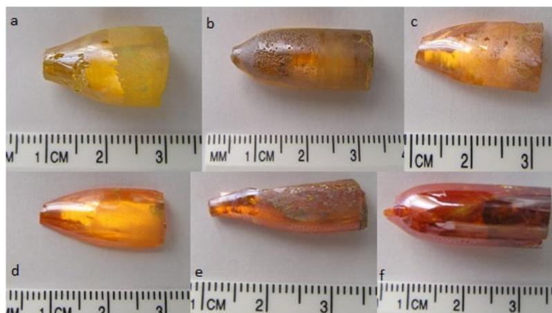
**Figure S2.** As-grown  $\text{TIPb}_2\text{Br}_{5-x}\text{I}_x$  single crystals: a –  $\text{TIPb}_2\text{Br}_3\text{I}_2$ , b –  $\text{TIPb}_2\text{Br}_{2.5}\text{I}_{2.5}$ , c –  $\text{TIPb}_2\text{Br}_2\text{I}_3$ , d –  $\text{TIPb}_2\text{Br}_{1.5}\text{I}_{3.5}$ , e –  $\text{TIPb}_2\text{BrI}_4$ , f –  $\text{TIPb}_2\text{Br}_{0.5}\text{I}_{4.5}$ .
