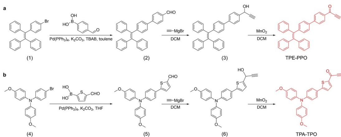
**Scheme S1.** Synthetic route of (a) TPE-BPO and (b) TPA-TPO
