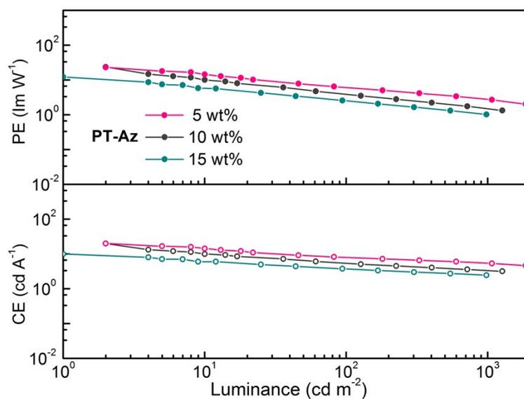
Figure S18 Power/Current Efficiency vs. Luminance relationships of PT-Az-based device.
