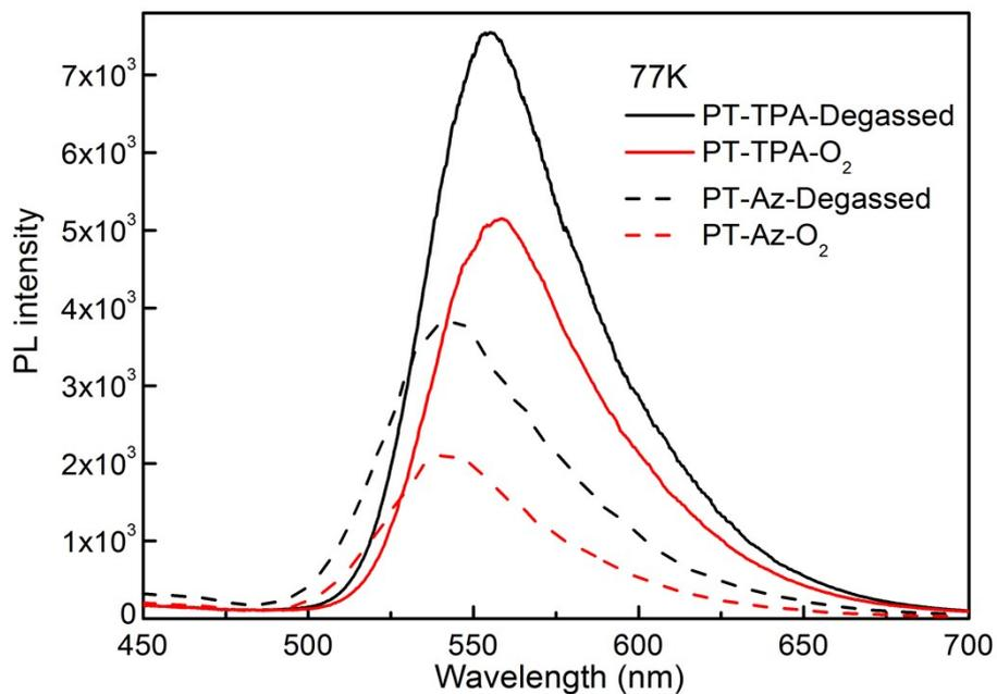
Figure S12 PL spectra of the toluene solutions ( $1.0 \times 10^{-5}$  M) of PT-TPA and PT-Az at 77K.
