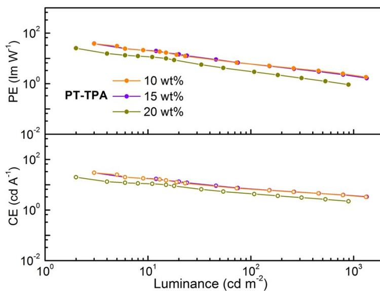
Figure S17 Power/Current Efficiency vs. Luminance relationships of PT-TPA-based device.
