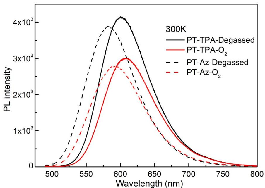
Figure S13 PL spectra of the toluene solutions ( $1.0 \times 10^{-5}$  M) of PT-TPA and PT-Az at 300K.
