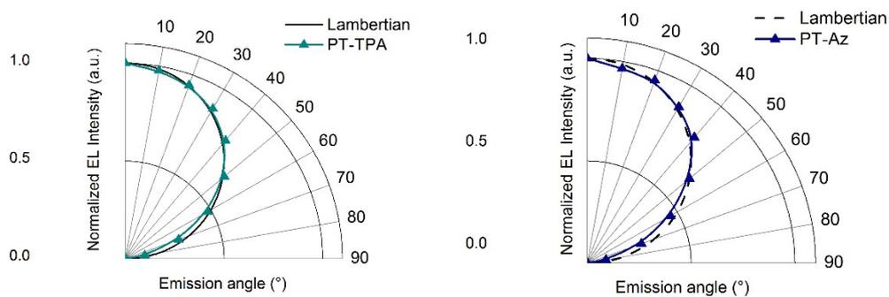
Figure S19 Angle-dependent EL emission pattern of the devices based on PT-TPA (left) and PT-Az (right). The black line is the Lambertian distribution.
