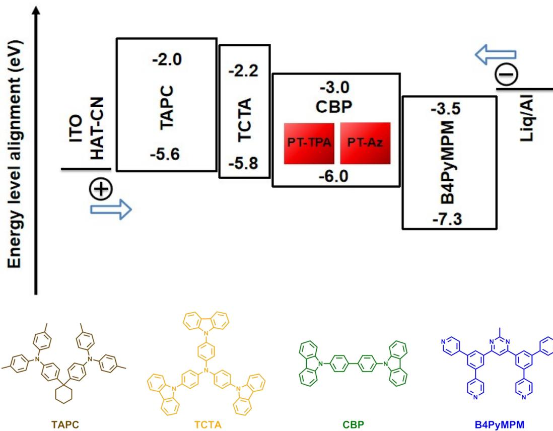
Figure S14 Energy level diagram and molecular structures of materials used in PT-TPA/PT-Az based device.
