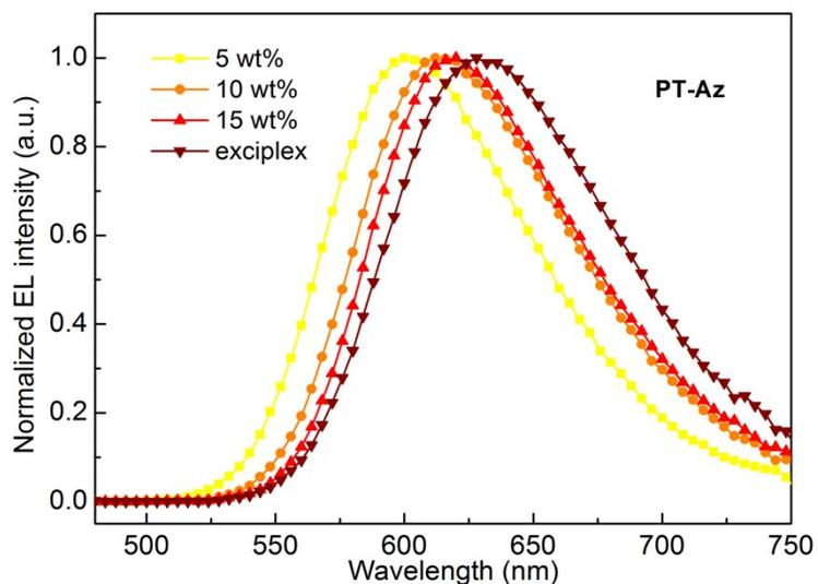
Figure S16 Electroluminescence (EL) spectra curve of PT-Az at  $0.1 \text{ mA cm}^{-2}$ .
