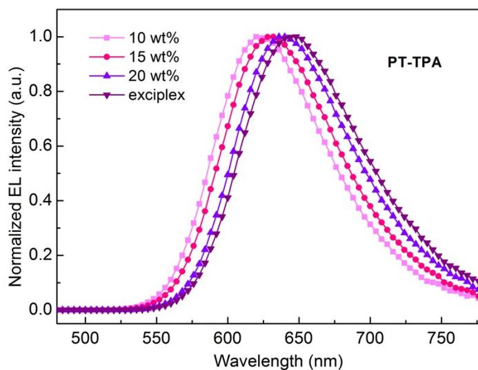
Figure S15 Electroluminescence (EL) spectra curve of PT-TPA at 0.1 mA cm<sup>-2</sup>.
