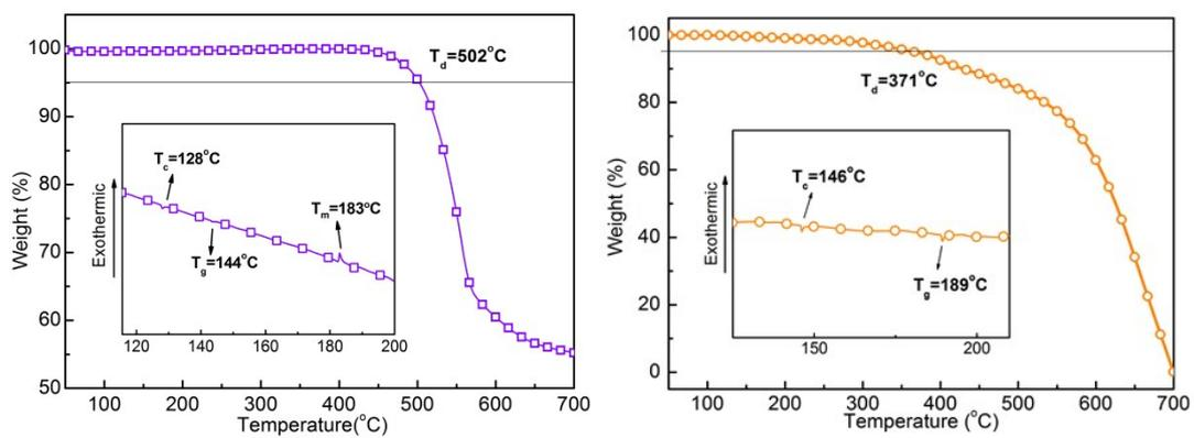
Figure S6 TGA and DSC (inset) curves of PT-TPA and PT-Az at a heating rate of 10 °C/min under nitrogen atmosphere.
