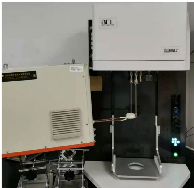
Figure S5. Set-up for measuring water vapor adsorption capacity of MF@MIL-1 when LECH was applied during the measurement.
