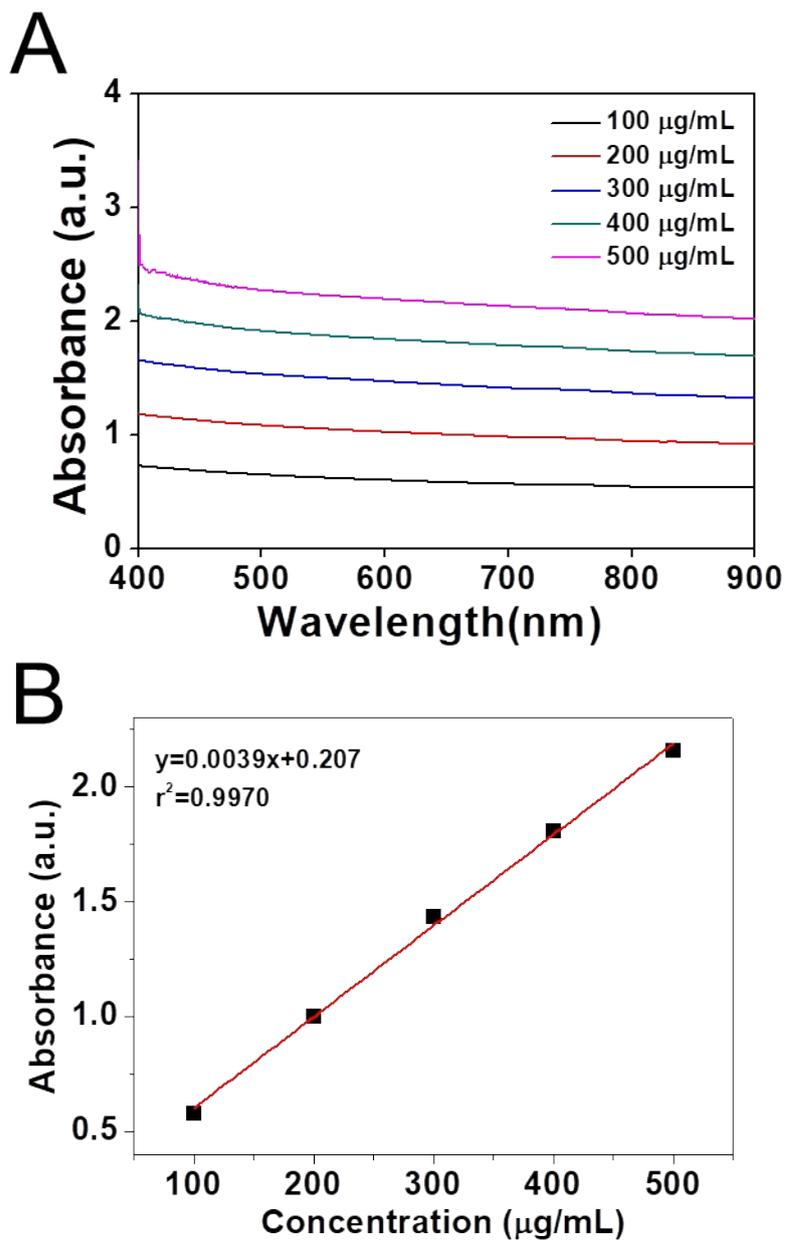
**Figure S10.** (A) UV-vis-NIR absorbance spectra of PEGylation NSH NSs dispersed in water at different concentrations. (B) Normalized absorbance intensity of PEGylation NSH NSs divided by the characteristic length of the cell ( $A/L$ ) at different concentrations for  $\lambda=808$  nm.
