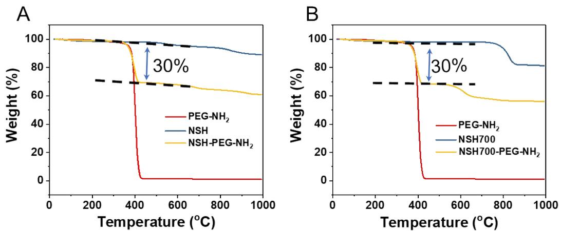
Figure S6. Thermogravimetric analysis (TGA) of NSH NSs, NSH700 NSs, and PEGylated NSH NSs and NSH700 NSs.
