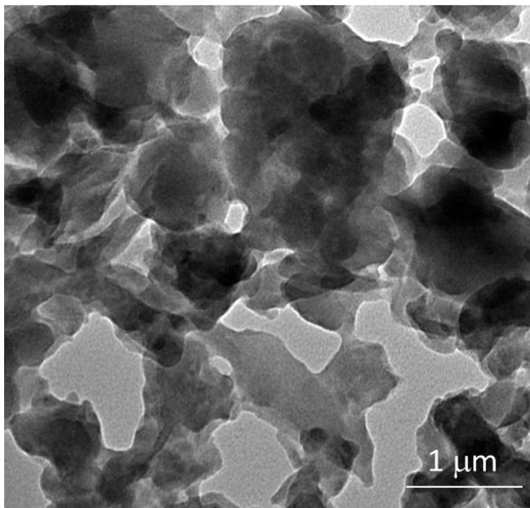
**Figure S1.** TEM images of NSH after wet grinding in NMP at 1000 rpm for 30 min.
