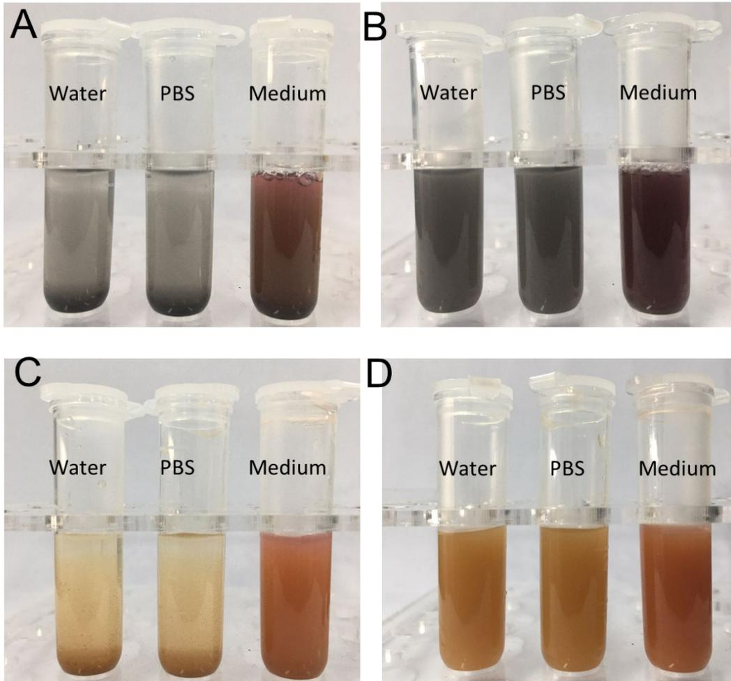
**Figure S7.** The distribution of (A) NSH NSs and (C) NSH700 NSs in water, PBS, and medium. The distribution of (B) PEGylation NSH NSs and (D) PEGylation NSH700 NSs in water, PBS, and medium.
