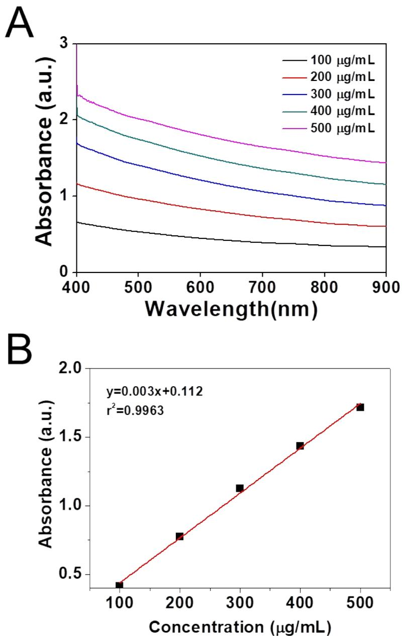
**Figure S9.** (A) UV-vis-NIR absorbance spectra of PEGylation NSH700 NSs dispersed in water at different concentrations. (B) Normalized absorbance intensity of PEGylation NSH700 NSs divided by the characteristic length of the cell ( $A/L$ ) at different concentrations for  $\lambda=808$  nm.
