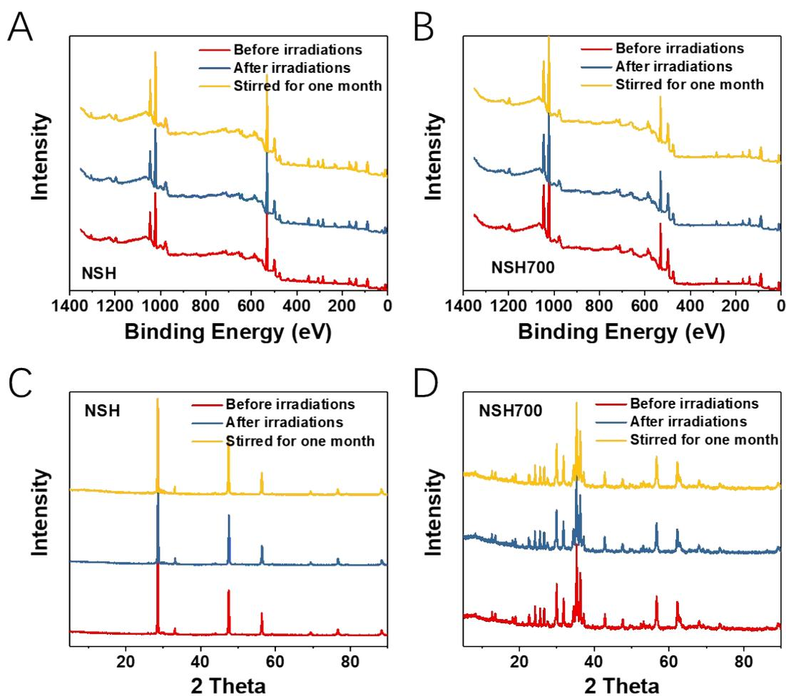
**Figure S8.** XPS spectra of fresh prepared, long-term stored, and laser and US irradiated (A) NSH NSs and (B) NSH700 NSs. XRD spectra of fresh prepared, long-term stored, and laser and US irradiated (C) NSH NSs and (D) NSH700 NSs.
