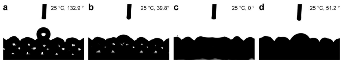
Fig. S9 Water contact angle corresponding to different fibers. (a) The CNT@PDMS coiled coaxial fiber. (b) The CNT@PDMS coiled coaxial fiber after oxygen plasma treatment. (c) The CNT@PDMS coiled coaxial fiber after polymerizing dopamine. (d) The MXene/SWCNTs-coated CNT@PDMS coiled coaxial fiber.
