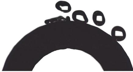
**Fig. S8.** The drop impact on curved fin-stripe non-wetting surface. The drop moves like the motion after the impact on flat fin-stripe non-wetting surface. The curvature of tested curved surface is  $0.1 \text{ mm}^{-1}$ , and Weber number of the impacting drop is 23.8.
