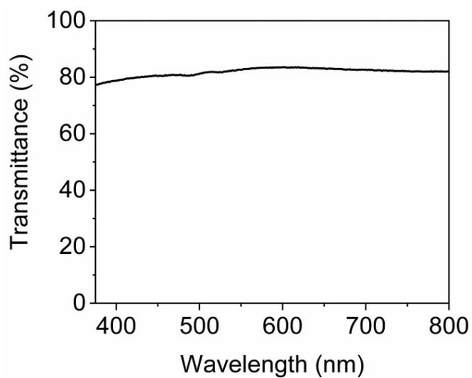
**Fig. S11.** Transmittance spectrum of a PDI@EC@PVA film loaded with AuNSs (0.02 wt%, thickness  $\sim 100 \mu\text{m}$ ), which demonstrates its high transparency to visible light.
