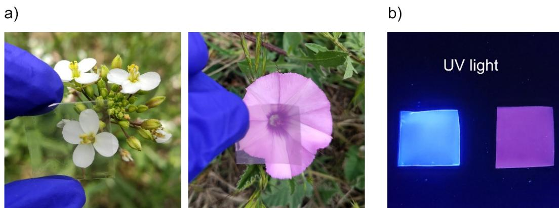
**Fig. S8.** Photographs taken (a) under ambient conditions and (b) under irradiation with a 365 nm UV lamp in the dark for two polymer films loaded with thermofluorochromic SLPs: (left) PDI/DCA@EC<sub>0.25</sub>OC<sub>0.25</sub>M812<sub>0.5</sub>@PVA and (right) PDI/DCA@EC<sub>0.3</sub>OC<sub>0.6</sub>M812<sub>0.1</sub>@PVA.
