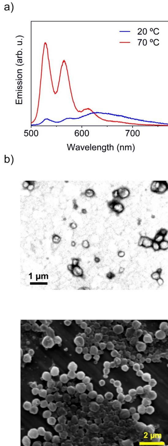
**Fig. S2.** a) Emission spectra of an aqueous suspension of PDI@OC\_SLPs acquired below (20 °C, blue) and above (70 °C, red) octacosane's melting point ( $\lambda_{\text{exc}} = 405 \text{ nm}$ ). The switch from excimer to pure monomer emission upon PCM melting can be clearly observed. b) TEM image of (top) PDI@EC\_SLPs (negative staining with uranyl acetate), and (bottom) SEM image of PDI@TC\_SLPs.
