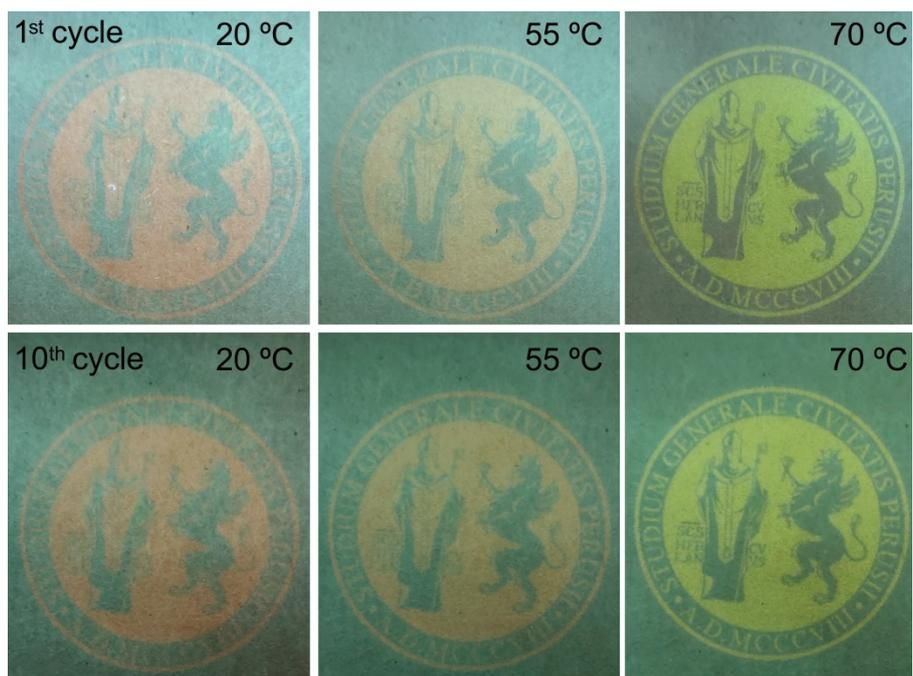
**Fig. S6.** Photographs of the emission from a paper inkjet-printed with a mixture of PDI@TC\_SLPs and PDI@OC\_SLPs. The thermofluorochromic sample was subjected to 10 consecutive heating-cooling cycles and images are shown for (top) the 1<sup>st</sup> and (bottom) 10<sup>th</sup> of these cycles. All the photographs were taken under wide field illumination with a 365 nm UV lamp.
