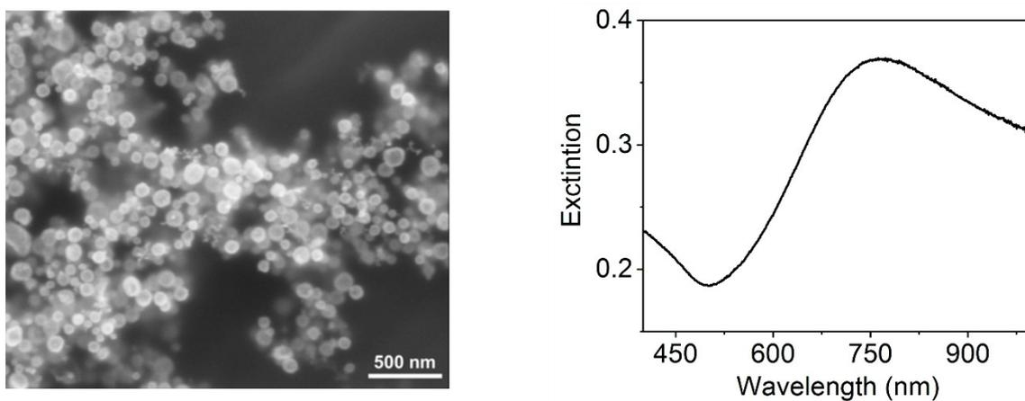
**Fig. S10.** SEM image and extinction spectra in water of the AuNSs ( $22 \mu\text{g mL}^{-1}$ ) used in this work as NIR-excitabile nanoheaters.
