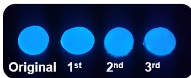
Fig. S10. Photographs of A_{4.75}\text{-}S_{0.25}\text{-}U_{16} hydrogels under a 365 nm UV lamp (from left to right: original sample, the 1st-3rd test were performed on the gels with 5 min, 10 min and 15 min of exposure to electric stimuli).
