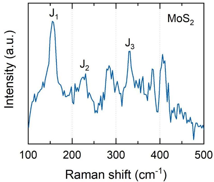
**Figure S1.** Raman spectrum of chemically exfoliated MoS<sub>2</sub>. Signatures from 1T MoS<sub>2</sub> are labeled as J<sub>1</sub>, J<sub>2</sub> and J<sub>3</sub> peaks at 156 cm<sup>-1</sup>, 226 cm<sup>-1</sup> and 333 cm<sup>-1</sup>.<sup>1,2</sup>
