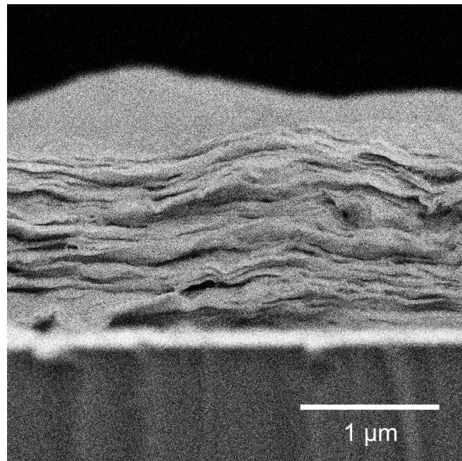
**Figure S4** A SEM cross sectional image of a representative restacked WS<sub>2</sub> film.
