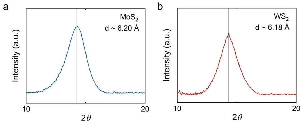
**Figure S5.** XRD of the toluene treated (a)  $\text{MoS}_2$  and (b)  $\text{WS}_2$ .
