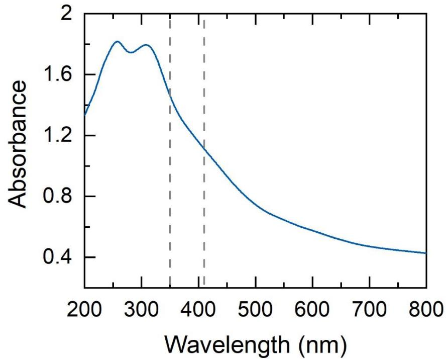
**Figure S2** UV-Vis spectrum of chemically exfoliated MoS<sub>2</sub>. The 70 % of 1T phase was determined by the extinction at 410 nm over 350 nm as well as the calibration curve in Ref 3.
