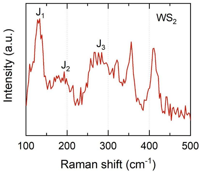
**Figure S3** Raman spectrum of chemically exfoliated WS<sub>2</sub>. Signatures from 1T WS<sub>2</sub> are labeled as J<sub>1</sub>, J<sub>2</sub> and J<sub>3</sub>.<sup>4</sup>
