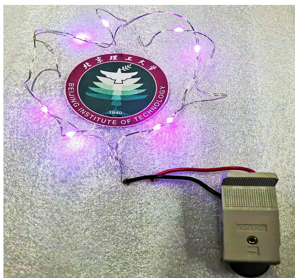
Fig. S18 Two Zn/C@poly(3-AP)/poly(4-AP)-2 cells with the mass loading of 21 \text{mg cm}^{-2} were connected in series to derive the purple LEDs.
