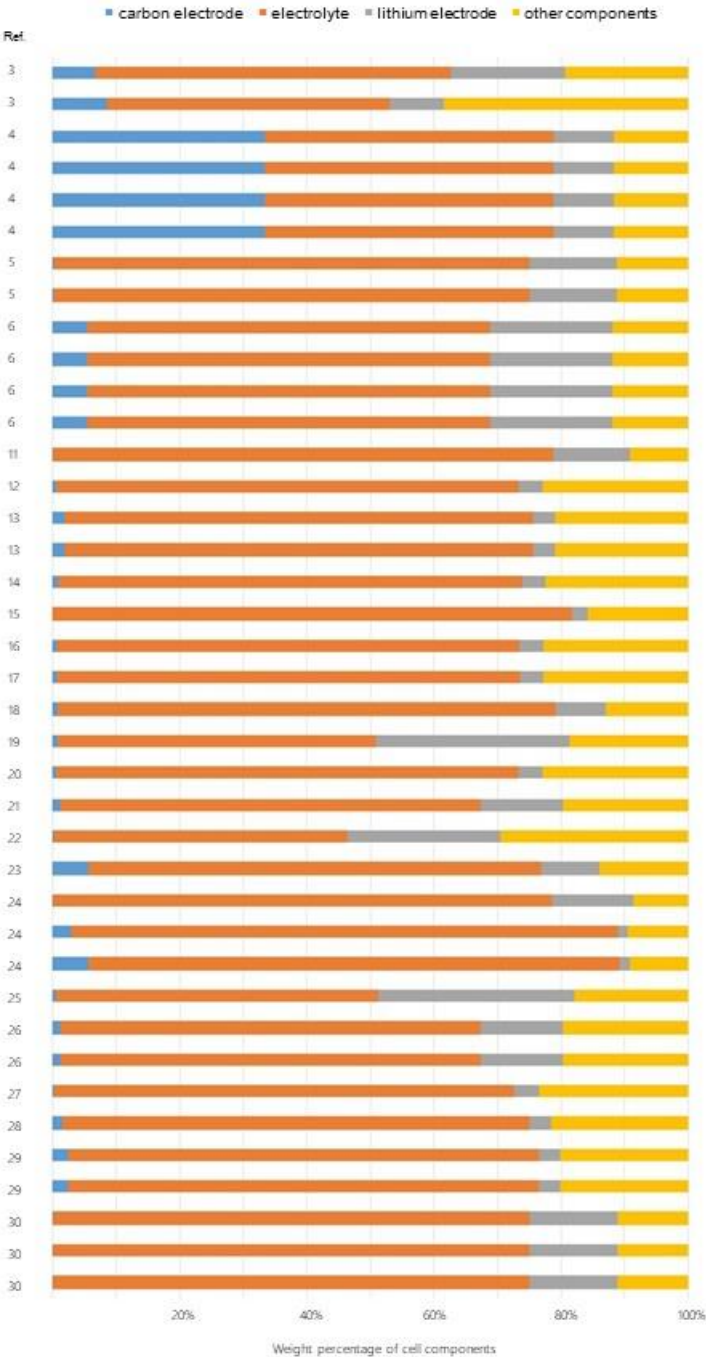
Figure S1 . Weight percentage of cell components in LABs used for energy density simulation
