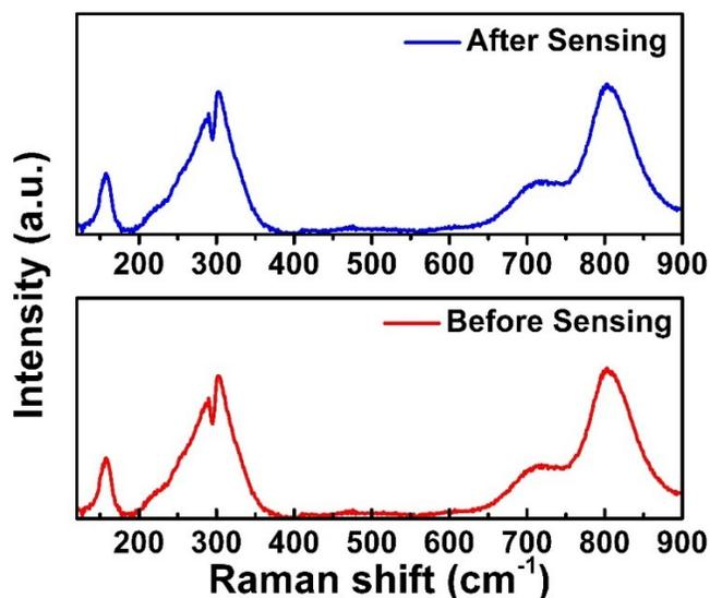
**Fig. S8** Raman spectra of  $\text{Bi}_2\text{WO}_6$  based pH sensor after and before sensing.
