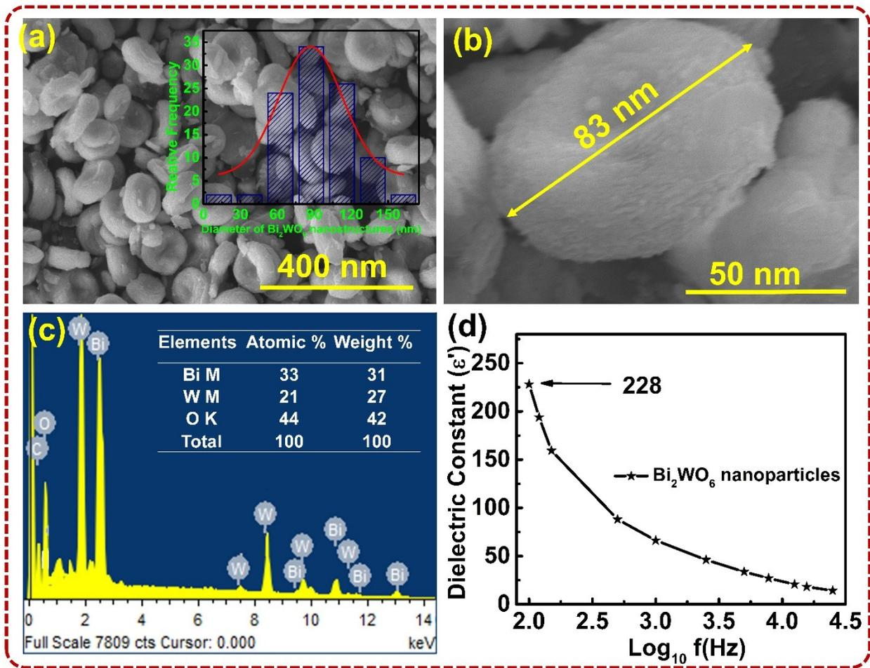
**Fig. S3.** (a) Low magnification FE-SEM micrographs and (inset) the Gaussian particle distribution of  $\text{Bi}_2\text{WO}_6$  nanoparticles (b) High resolution FE-SEM image of  $\text{Bi}_2\text{WO}_6$  nanoparticles. (c) elemental analysis of  $\text{Bi}_2\text{WO}_6$  nanoparticles (d) Variation of dielectric constant with respect to frequency of  $\text{Bi}_2\text{WO}_6$  nanoparticles.
