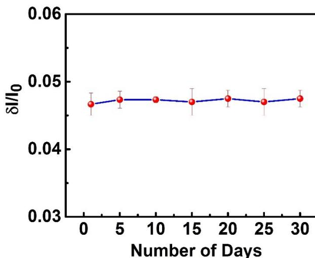
**Fig. S7** Normalized response of Bi<sub>2</sub>WO<sub>6</sub> based pH sensor for 30 days (N = 5).
