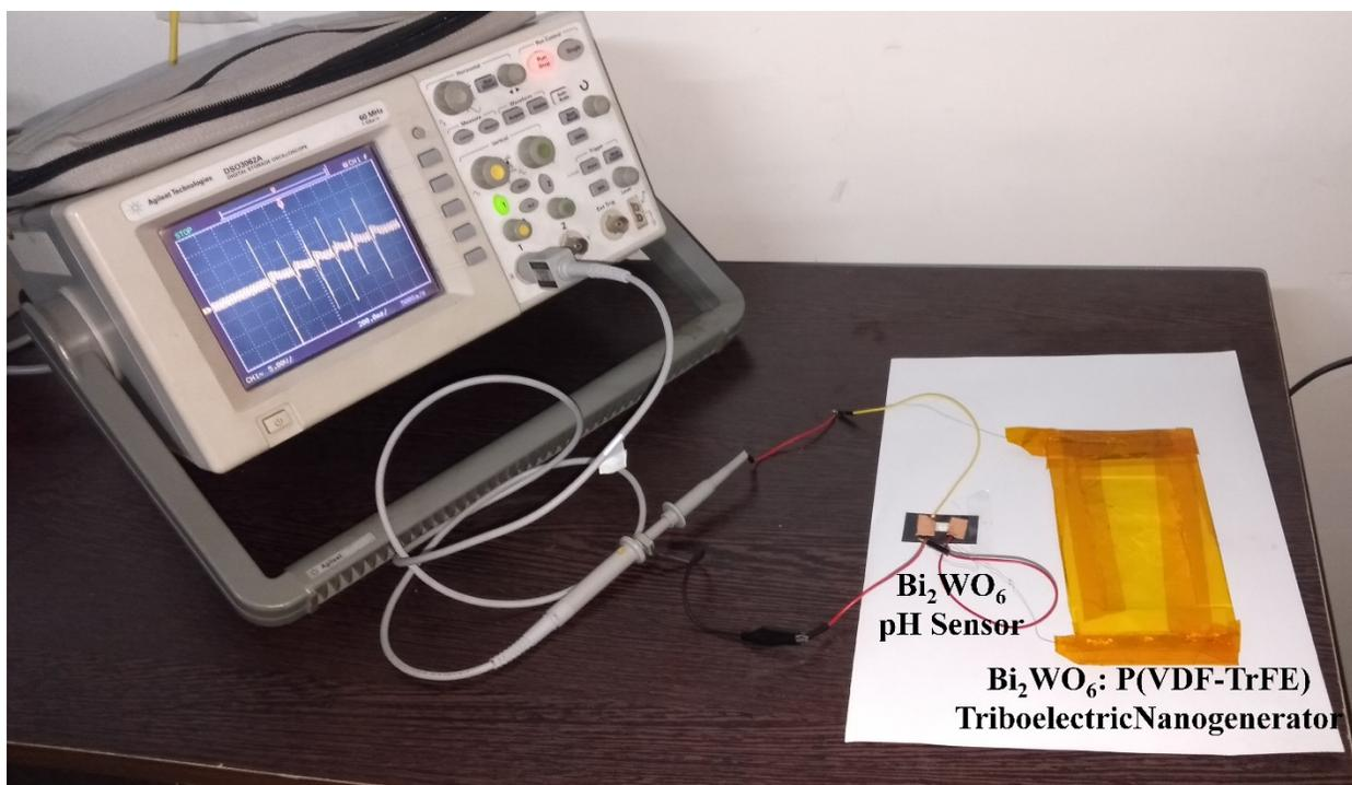
**Fig. S6.** Pictorial representation of self-power Bi<sub>2</sub>WO<sub>6</sub> based pH sensor.
