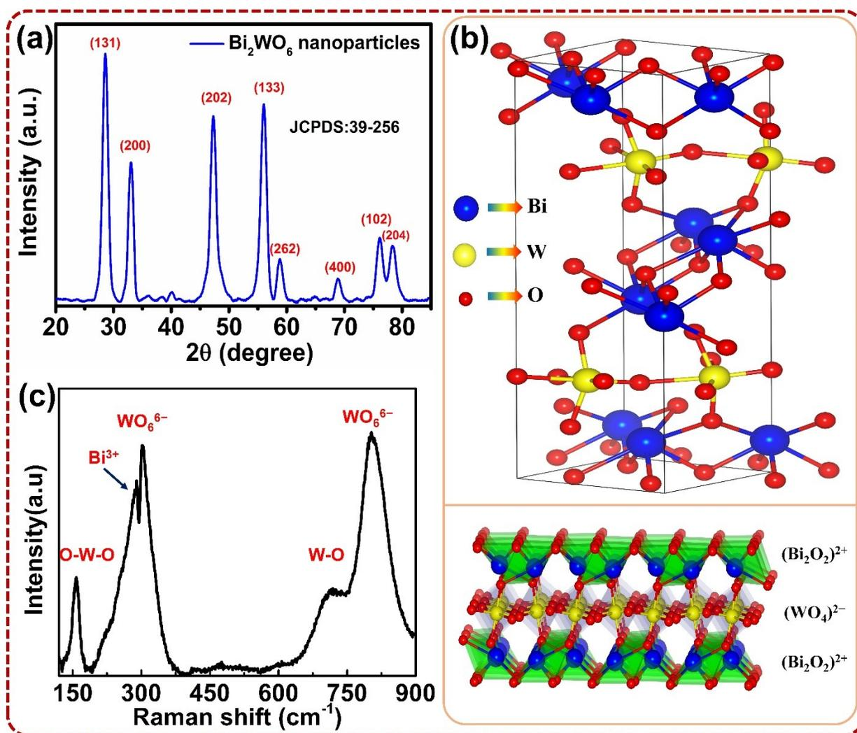
**Fig. S2.** (a) X-ray diffraction (b) layered like structure of orthorhombic  $\text{Bi}_2\text{WO}_6$ . (c) Raman spectra of  $\text{Bi}_2\text{WO}_6$  nanoparticles
