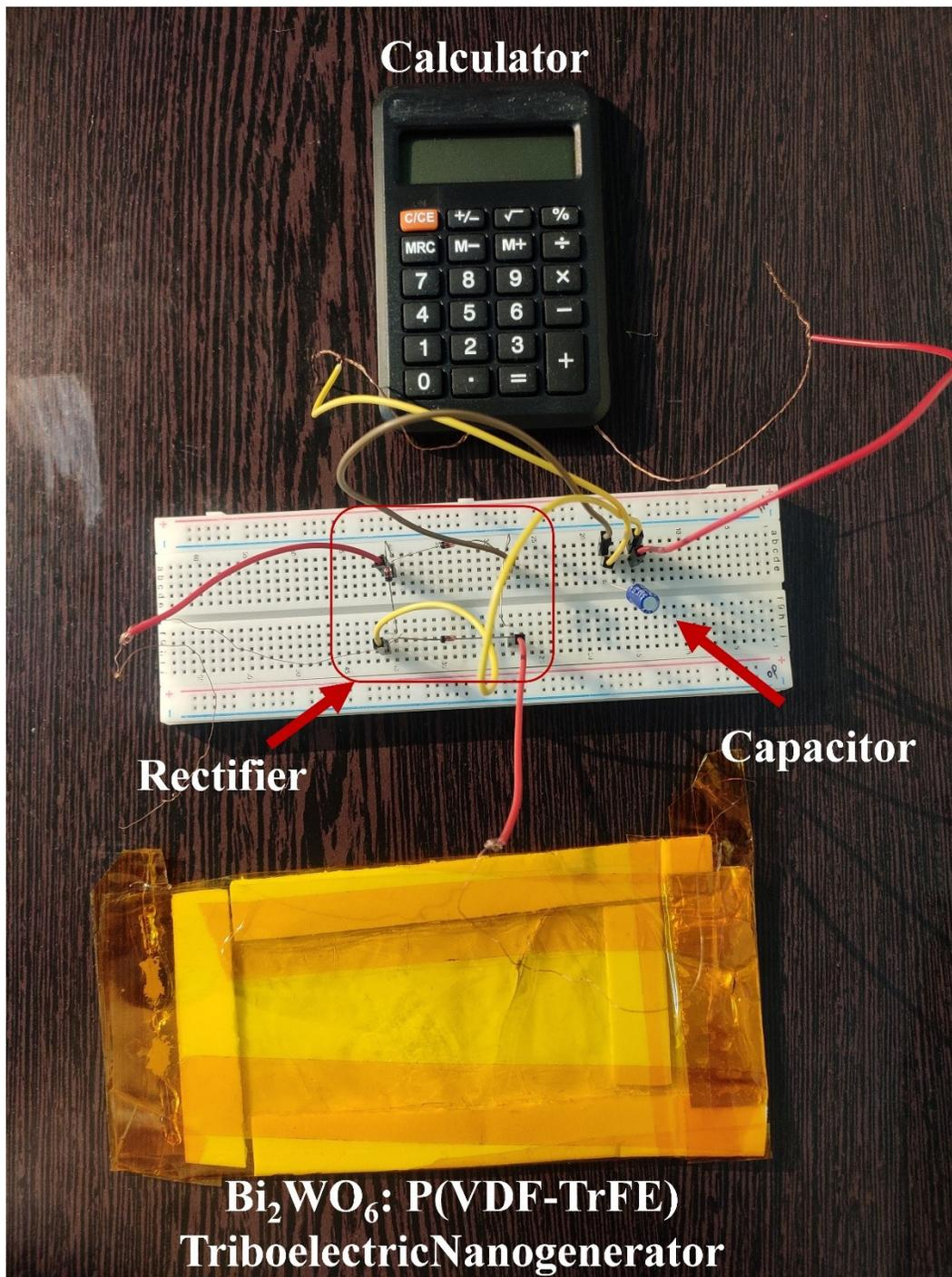
**Fig. S10.** Pictorial representation of rectification, charging of capacitor and powering of calculator using  $\text{Bi}_2\text{WO}_6$ : P(VDF-TrFE) triboelectric nanogenerator.
