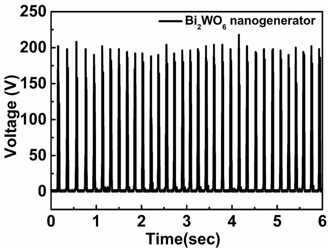
**Fig. S9.** Rectified output response of Bi<sub>2</sub>WO<sub>6</sub>: P(VDF-TrFE) triboelectric nanogenerator.
