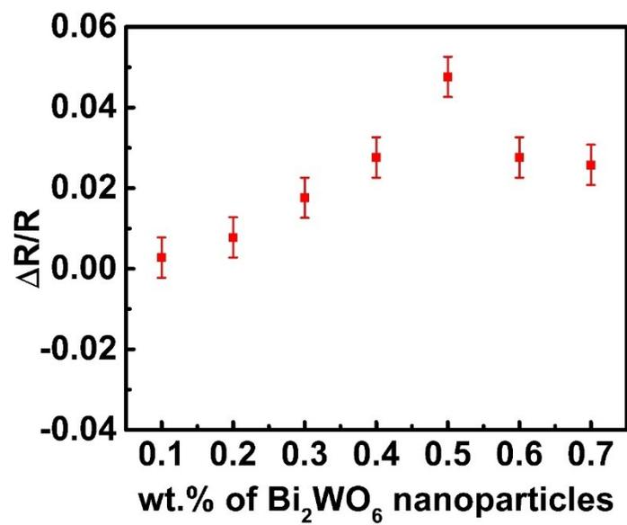
**Fig. S1.** Response of the  $\text{Bi}_2\text{WO}_6$  based pH sensor with the solution of pH-6.
