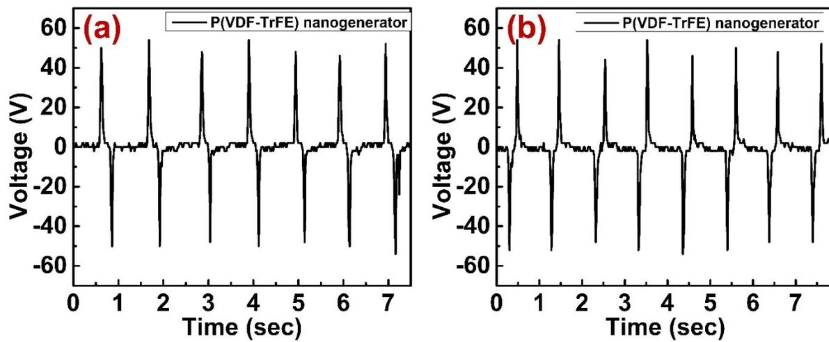
Fig. S5. Output voltage of P(VDF-TrFE) triboelectric nanogenerator under (a) forward connection and (b) reverse connection condition.
