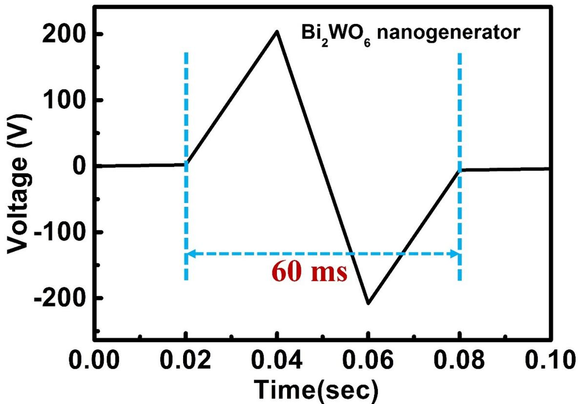
Fig. S4. Response time of Bi<sub>2</sub>WO<sub>6</sub>: P(VDF-TrFE) triboelectric nanogenerator.
