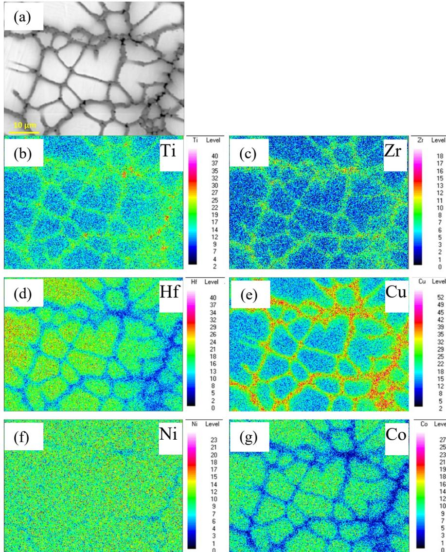
Figure S2 SEM image of the as-cast Co16.7 HEI, shows a single phase with a grain size of around 10 μm, and neither secondary phase or precipitation was found. The corresponding elemental mapping of Ti (b), Zr (c), Hf (d), Cu (e), Ni (f) and Co (g).
