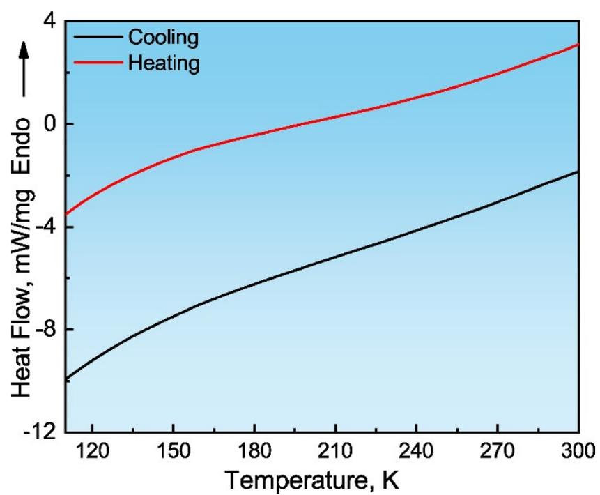
Figure S5 DSC heating and cooling curves of the Co<sub>16.7</sub> HEI in the temperature range from 300 to 110 K.
