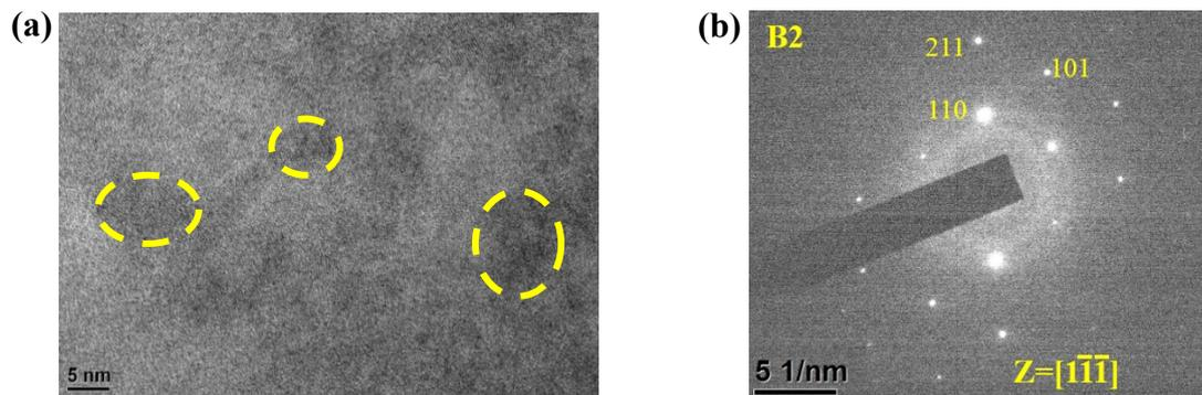
Figure S3 TEM image (a) and the corresponding selected area electron diffraction (SAED) pattern (b) of the  $\text{Co}_{16.7}$  HEI. Single-phase with a B2 structure was confirmed while nano-scale chemical heterogeneity was also seen based on nano-scale contrast.
