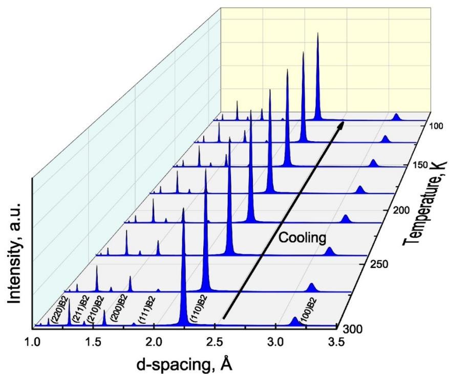
Figure S4 Evolution of the diffraction patterns during cooling from room temperature to 93 K. No change in the peak intensity was observed, indicating that the B2-phase keeps unchanged during the cooling process.
