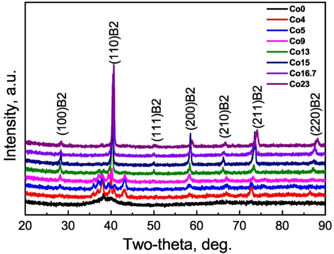
Figure S1 X-ray diffraction pattern of  $(\text{TiZrHfCuNi})_{100-x}\text{Co}_x$  alloys (a), alloys with  $x > 15$  show different peaks of a single B2 structure.
