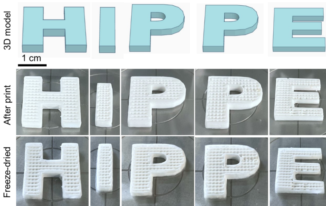
Fig. S5 3D printed letters demonstrating the print quality in wet condition and shrinkage of the structure after freeze-drying. The scale bar is 1 cm.
