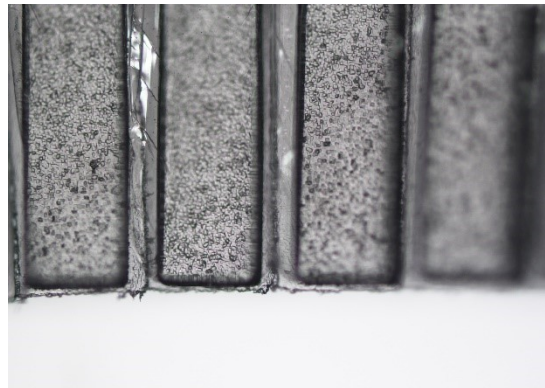
Figure S9: Degradation test: top left test specimen 17 mm x 6 mm x 0.2 mm, with 0.5 mm wide comb tooth; top right before ageing; bottom left after ageing with PBS and bottom right ageing with hydrogen peroxide.
