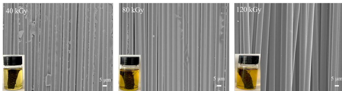
Figs. S33. Photographs and SEM images of the recycled CF at different irradiation doses.
