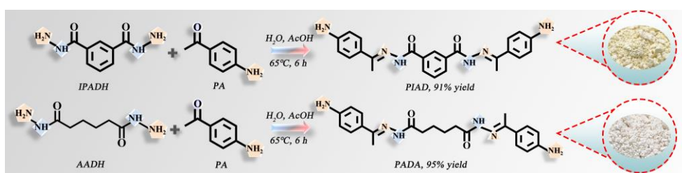
Figs. S1. Synthetic route of \gamma -ray-responsive curing agents PIAD and PADA.
