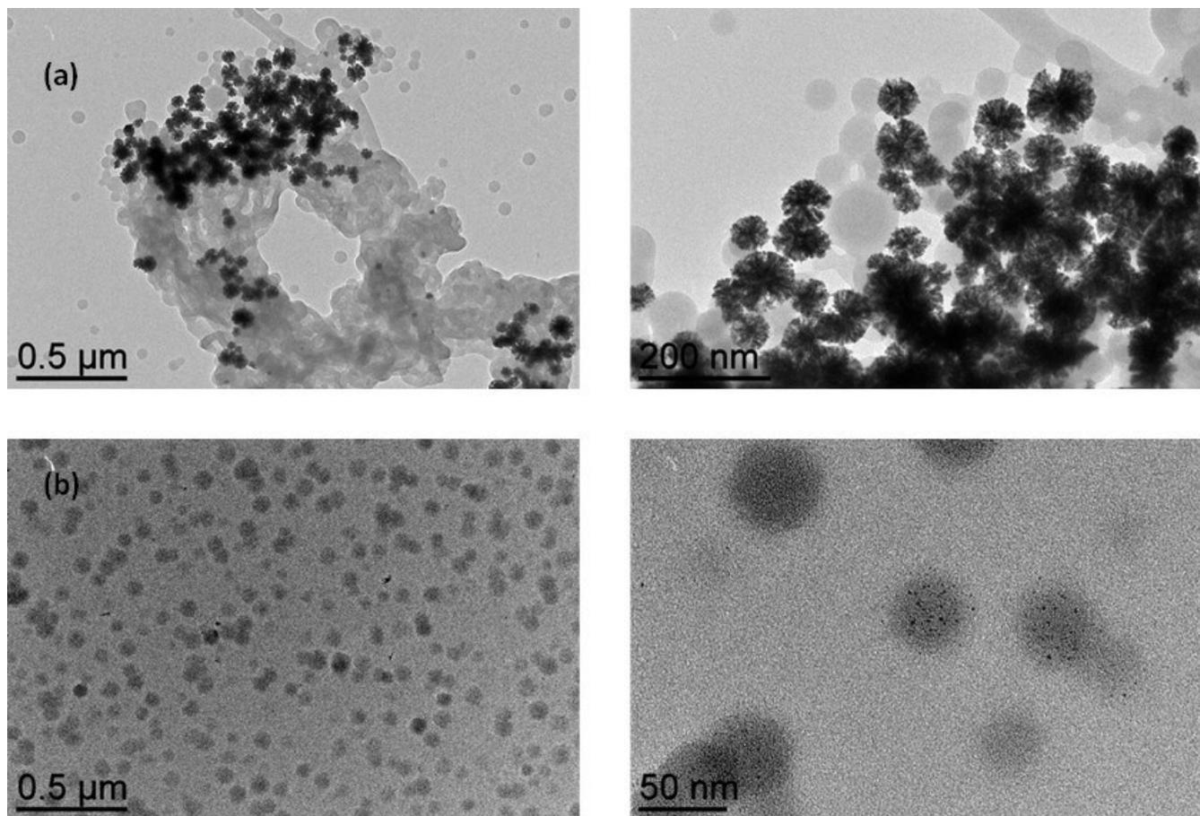
Figure S3. TEM images of the **CCM-N-0.2** polymer latex after loading with  $[\text{RhCl}(\text{COD})]_2$  and reduction with  $\text{H}_2$  (20 bar) in the presence of  $\text{NEt}_3$  (5 equiv. per Rh) for 20 h. (a) P/Rh = 1, 25°C. (b) P/Rh = 4, 60°C.
