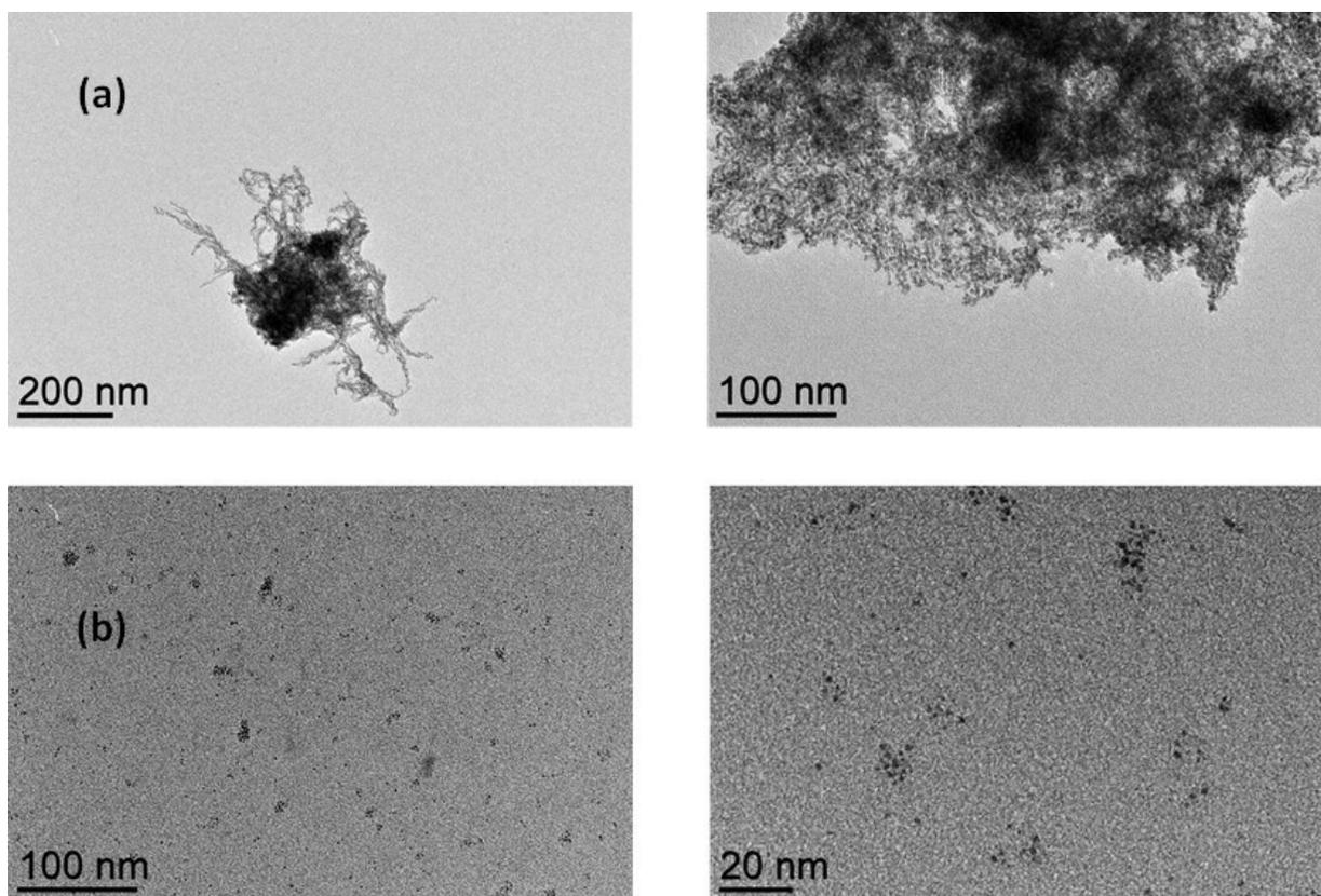
Figure S4. TEM images of the Rh NPs obtained from a toluene solution of  $[\text{RhCl}(\text{COD})]_2$  in the presence of  $\text{PPh}_3$ ,  $\text{H}_2$  (20 bar) and  $\text{NEt}_3$  (5 equiv per Rh). (a) P/Rh = 1:1, T = 25°C. (b) P/Rh = 4:1, 60°C.
