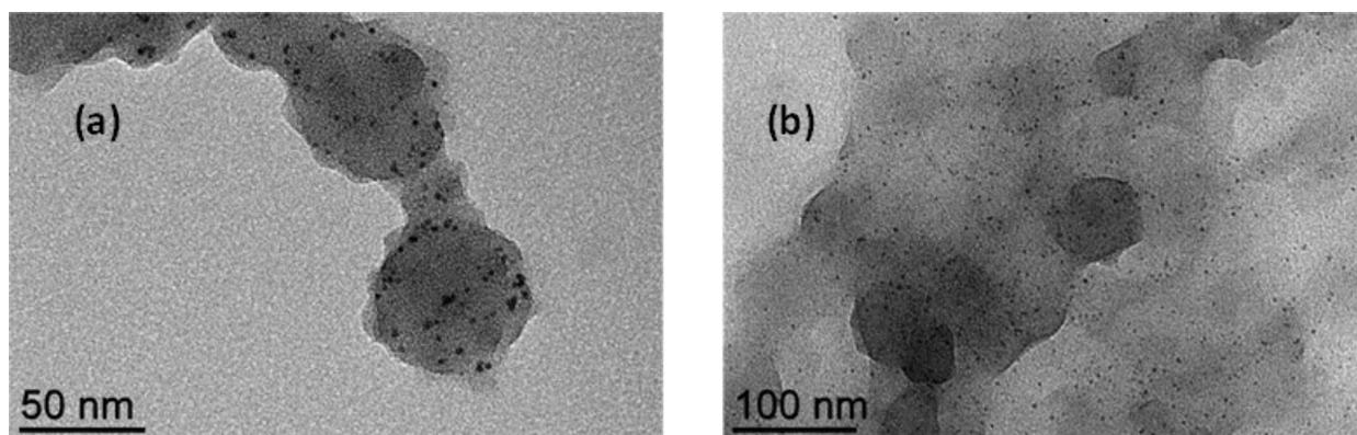
Figure S5. TEM images of Rh NP@(CCM-C 0.1) obtained with P/Rh = 1:1 and reduction with  $\text{H}_2$  (20 bar) at 25°C for 20 h with different  $\text{NEt}_3/\text{Rh}$  ratios: (a) 0; (b) 1 (an image corresponding to  $\text{NEt}_3/\text{Rh} = 5$  is available in Figure 3 (a)).
