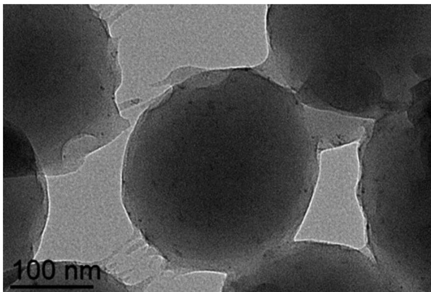
Figure S2. TEM image of the Rh NP@(CCM-N-0.1) obtained from a 25% loaded latex (P/Rh = 4) without added base at 90°C for 20 h.
