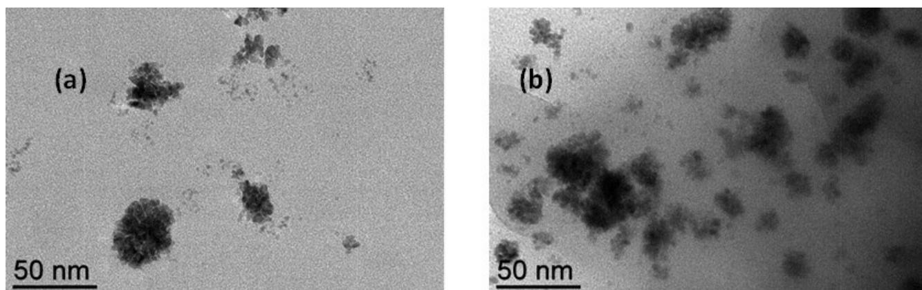
Figure S6. TEM images of Rh NP@(macroRAFT-C) obtained by  $[\text{RhCl}(\text{COD})]_2$  reduction with  $\text{H}_2$  (20 bar) at  $60^\circ\text{C}$  in methanol in the presence of  $\text{NEt}_3$  (10 equiv. per Rh) for 20 h. (a)  $4\text{VPMe}^+\text{I}^-/\text{Rh} = 4.7$  (equivalent to the experiment with CCM-C 0.1 at P/Rh = 1). (b)  $4\text{VPMe}^+\text{I}^-/\text{Rh} = 18.8$  (equivalent to the experiment with CCM-C 0.1 at P/Rh = 4).
