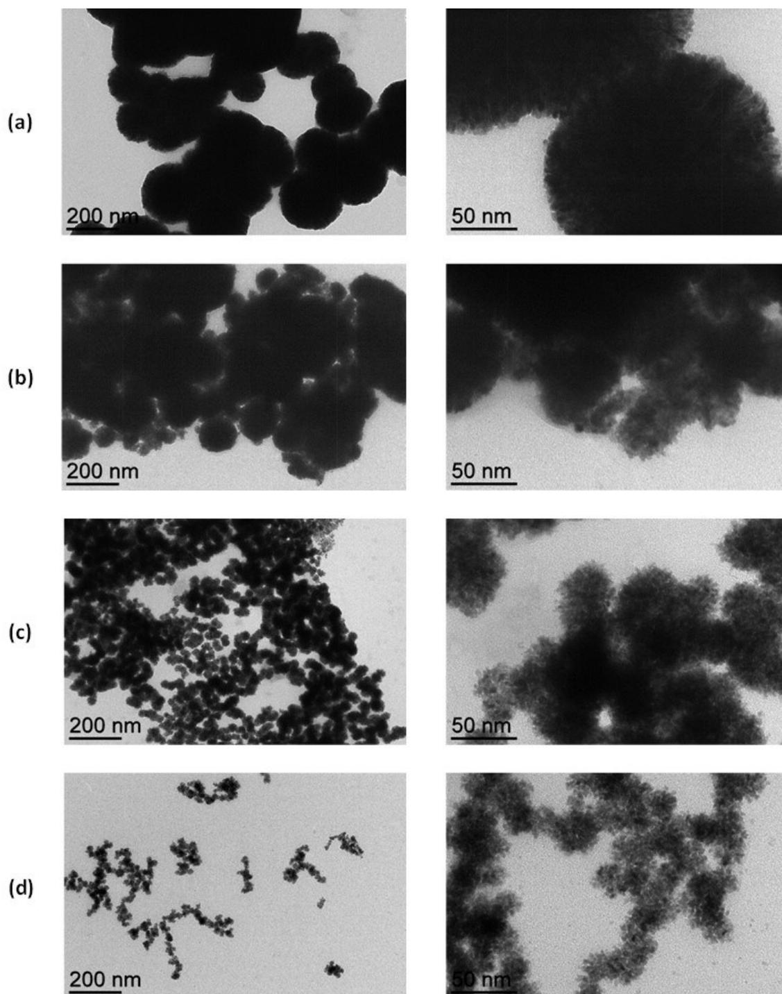
Figure S1. TEM images of the Rh NPs obtained from a toluene solution of  $[\text{RhCl}(\text{COD})]_2$  in the presence of PEOMA ((a) and (b) or **macroRAFT-N** ((c) and (d)),  $\text{H}_2$  (20 bar) and  $\text{NEt}_3$  (10 equiv per Rh) at  $60^\circ\text{C}$ . (a) and (c): PEOMA/Rh = 0.5:1. (b) and (d): PEOMA/Rh = 2:1.
